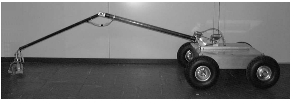
Figure 3: The Slugbot: a proof-of-concept robot predator
