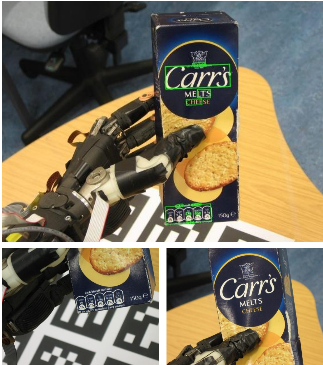
Figure 7.4: The TCZ strategy in action - the top image shows the text quadrilaterals identified at the first pose. Initially 10 (pose, zoom) pairs are generated, one for each quadrilateral. These are pruned back to 2 (pose, zoom) pairs which can each see half of the quadrilaterals, and the bottom two images were obtained from those (pose, zoom) pairs.
