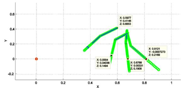
Figure 1. Using several fixed arm positions, all the possible arm angles could be determined to find the extents of the dressing trajectory. The reference frame origin for Baxter is at  $X,Y=(0,0)$ , several arm poses of the mannequin are shown projected onto the XY plane (plan view).
