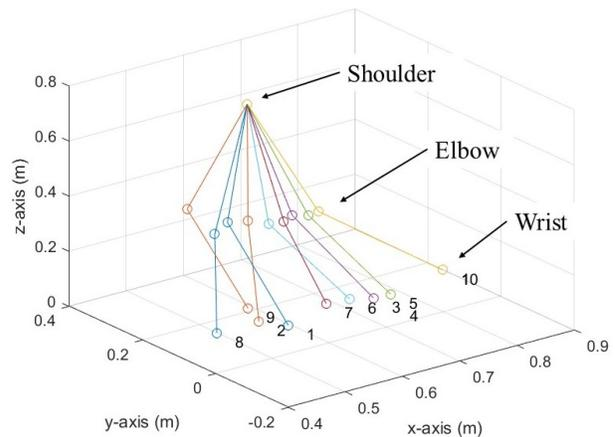
Figure 4. Mannequin arm poses (1-10) used for trajectory planning.
