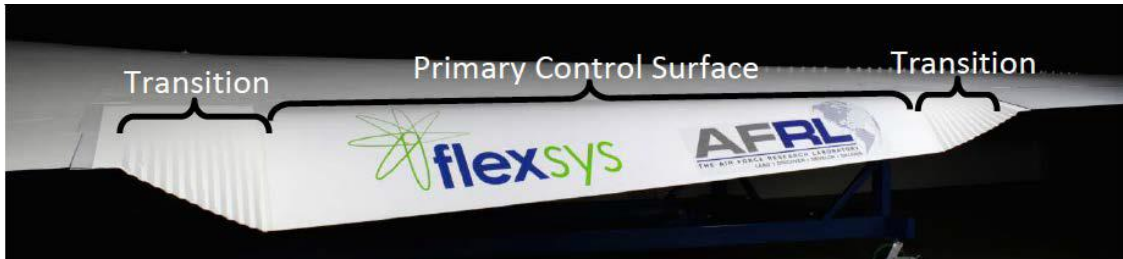
Fig.1 Morphing flap on Gulfstream III business jet, showing non-smooth transition surfaces [9].
