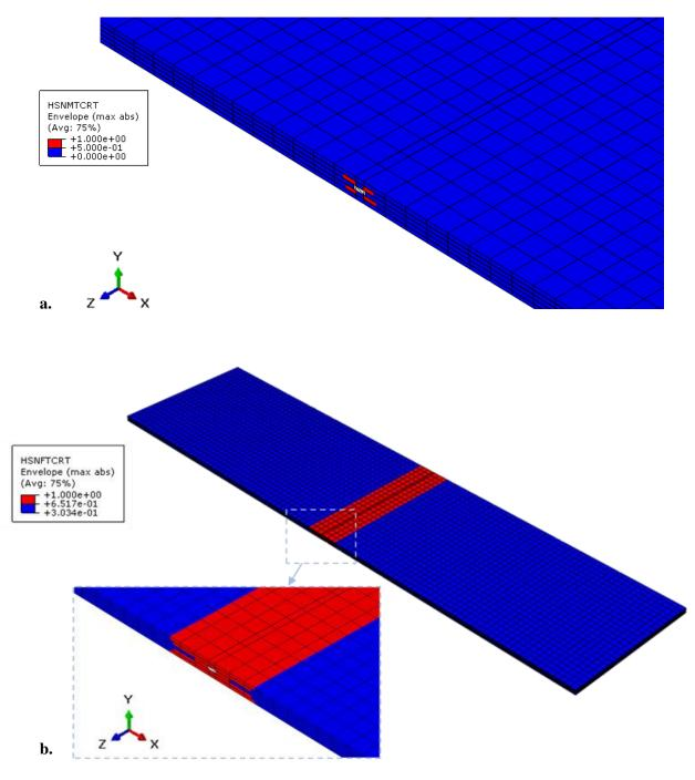
Figure 16. a) Hashin's matrix and b) Hashin's fibre tensile failure pattern at the ultimate failure stress (1578 MPa)
