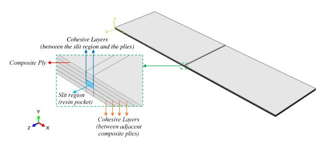
Figure 4. Partitions for the TCT specimen FE model
