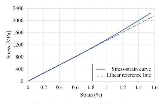
Figure 6. Stress-strain curve of non-slit [0]<sub>5</sub> specimen
