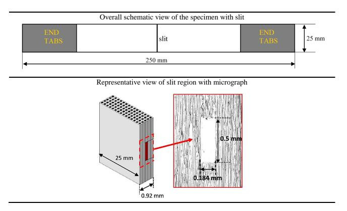
Figure 2. Schematic views of slit in TCT specimens
