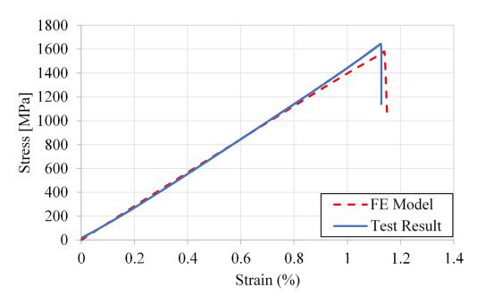
Figure 8. Comparison between a tension test and FE model for TCT [0]<sub>5</sub>-specimen.
