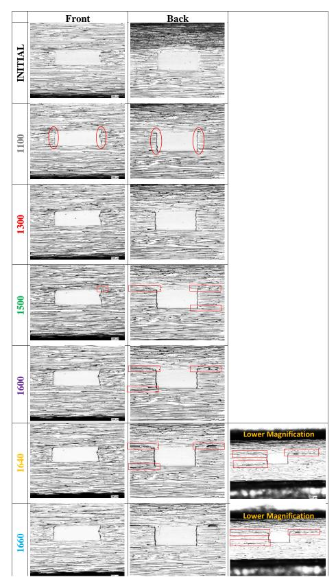
Figure 11. Damage progression in slit-specimen
