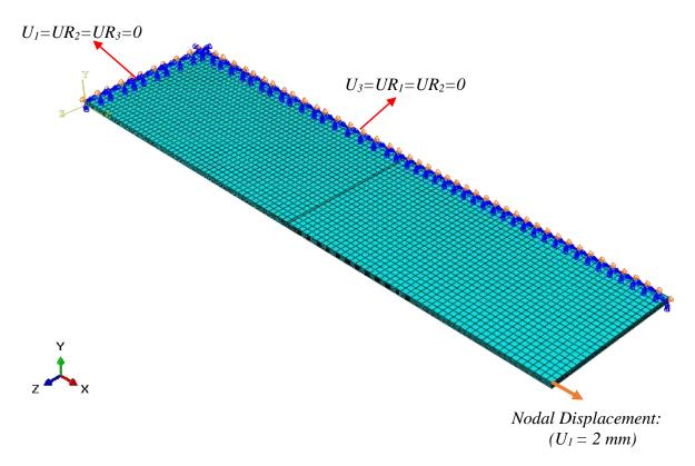
Figure 5. Mesh structure and assigned boundary conditions
