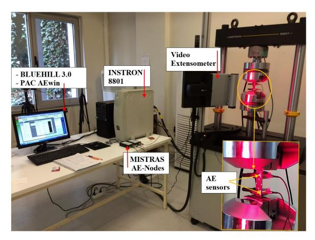
Figure 3. Tension test setup
