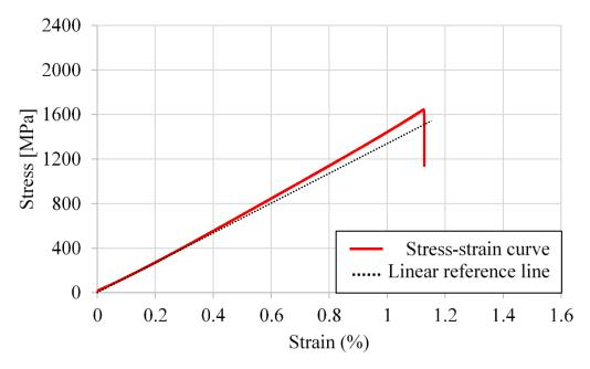
Figure 7. TCT stress-strain curve of TCT [0]<sub>5</sub> specimen.
