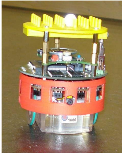
Fig. 1. An e-puck with Linux board fitted between the e-puck motherboard (lower) and the e-puck speaker board (upper). Note both the red skirt and the yellow hat that provides a matrix of pins for the reflective spheres which allow the tracking system to identify and track each robot.
