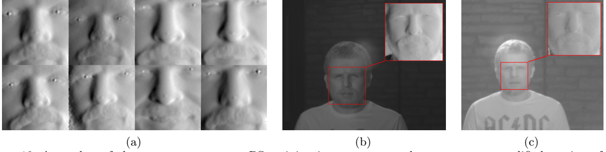
Figure 12. A number of close-range, two source PS training images were used to augment a modified version of the Photoface database, 31 a representative selection of which are shown in (a). We then test the usability of long-range 3D data to recognise known faces, using the recognition strategy of Hansen and Atkinson 30 and input data garnered from images taken at 10 m (b) and 15 m (c). In both cases, the system was able to successfully identify the subject from the long-range images.
