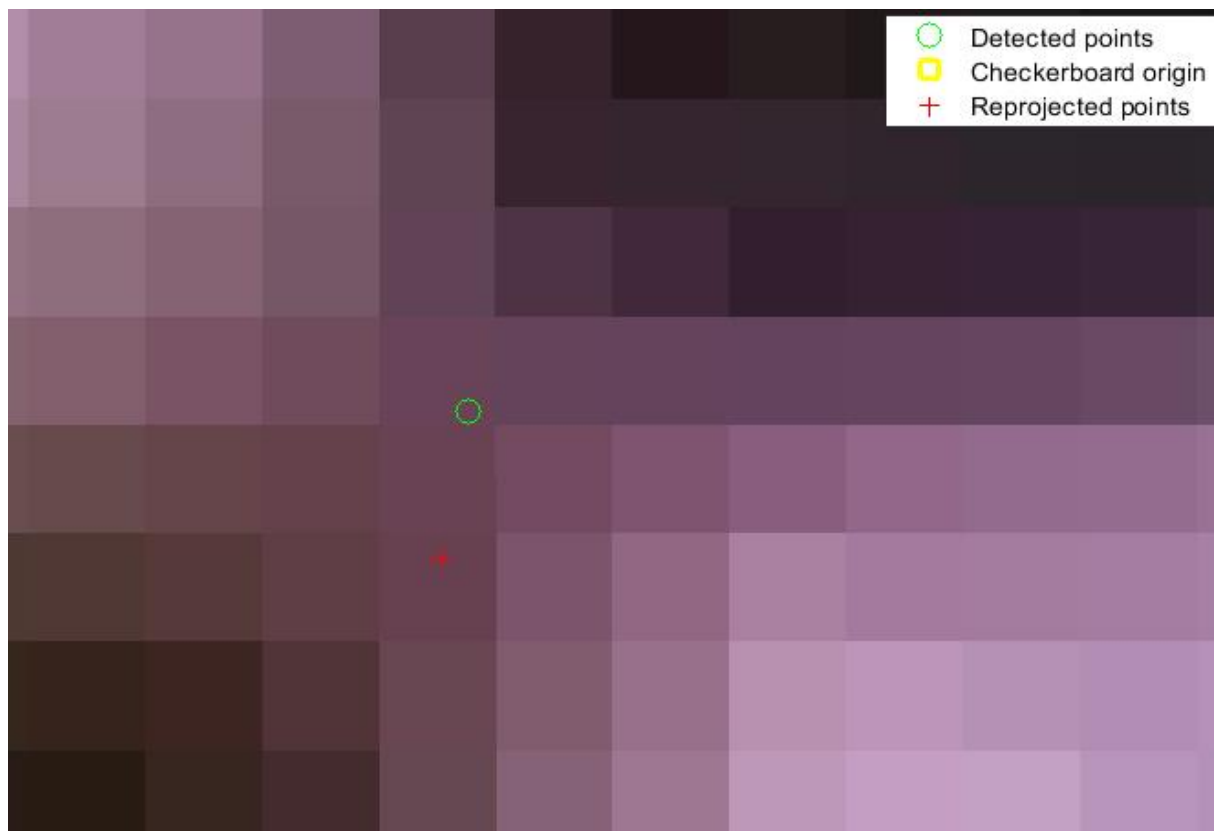
Figure 7.13: Reprojection error is the offset from the circle center to the cross intersection
