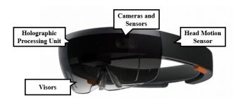
Figure 2. The mixed reality device HoloLens.
