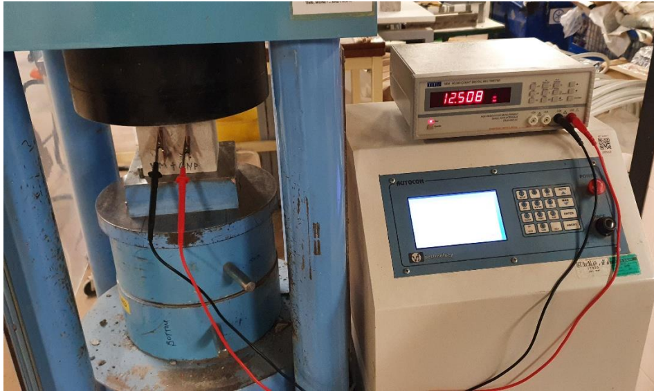
643 Figure 1. Typical sample setup for electrical resistivity response measurement under compressive 644 stress.
