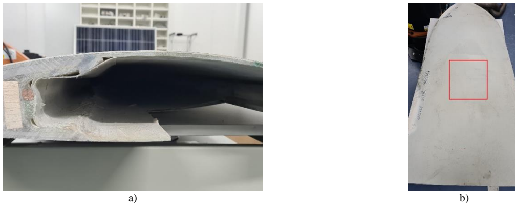
Figure 1. Eolic blade employed for the inspection. a) cross-section, b) highlighted delamination defect
