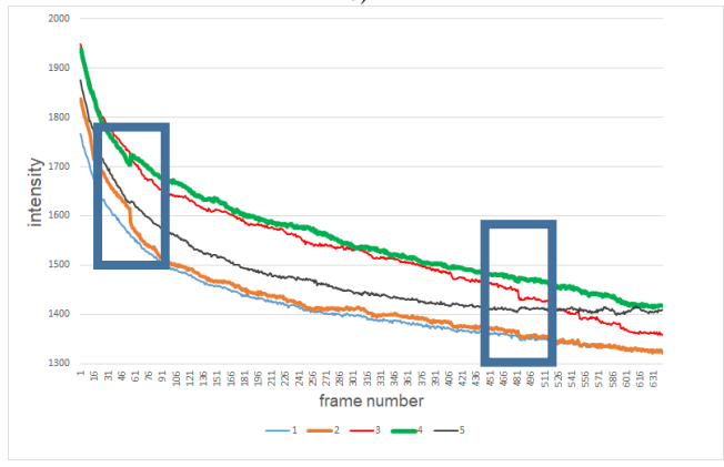
Figure 11. Phase image distortion in edges caused by overfit in registration. a and c) horizontal phase delta profiles with phase highlighted, b and d) thermogram of points in the distorted area, FBH corner points, 2 and 4, magnify the artifact derived from the overfit
