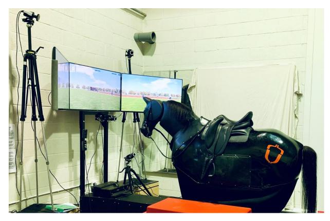
**Figure 3.3.** The riding simulator in Arena Mode with standard saddle and motion capture cameras. Not pictured: motion capture cameras placed to the rear and left side of the simulator.
