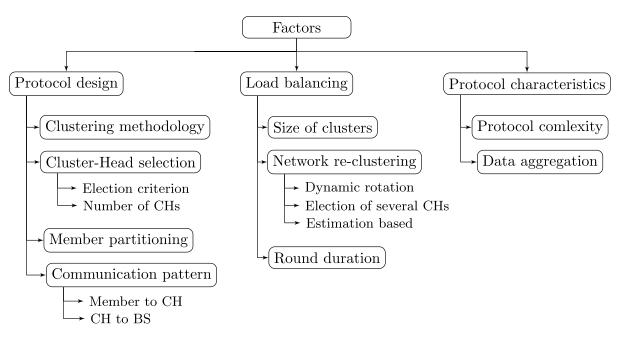
FIGURE 4. Taxonomy of factors influencing the energy efficiency of clustering protocols in WSNs.
