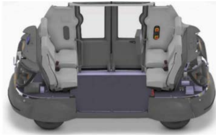
Figure 4. Cutaway of LSAV seating arrangement. Photo credit: Westfield Technology Group.
