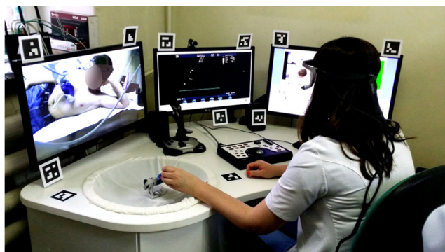
Fig. 7 Setup of eye tracking study for remote examination. Doctor controls the robot with the ReMeDi interface and wears a mobile eye tracker during the examination
