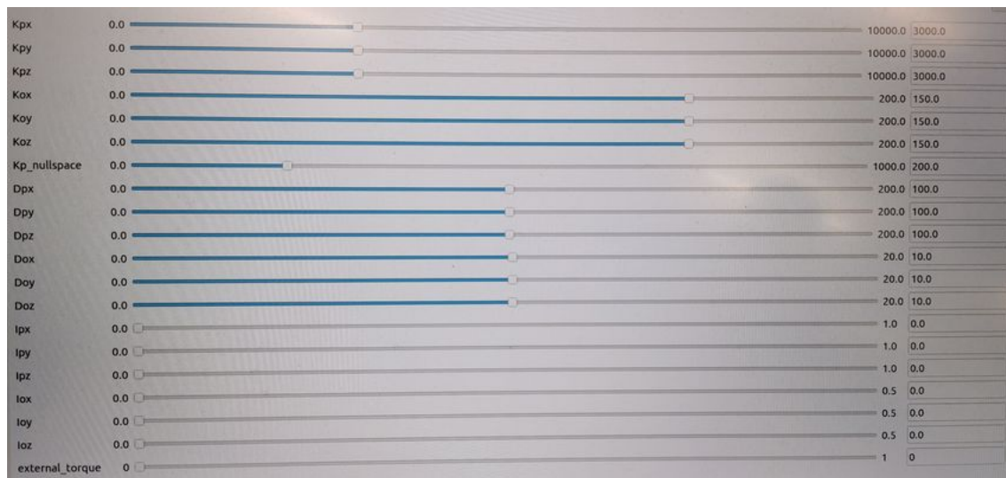
Figure 7.5: The GUI for the control system. The human operator can modify the parameters of the controller online to adjust the compliant behaviour, such as the stiffness and damping of the impedance controller etc.
