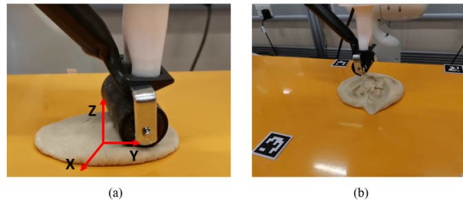
Figure 5.5: (a) The robot rolls the pizza dough with proper force and motion. (b) The robot interacts with the soft dough with a large force, so the roller gets stuck. In this case, the forces along the X and Y axes are too large, which means that the task has failed.
