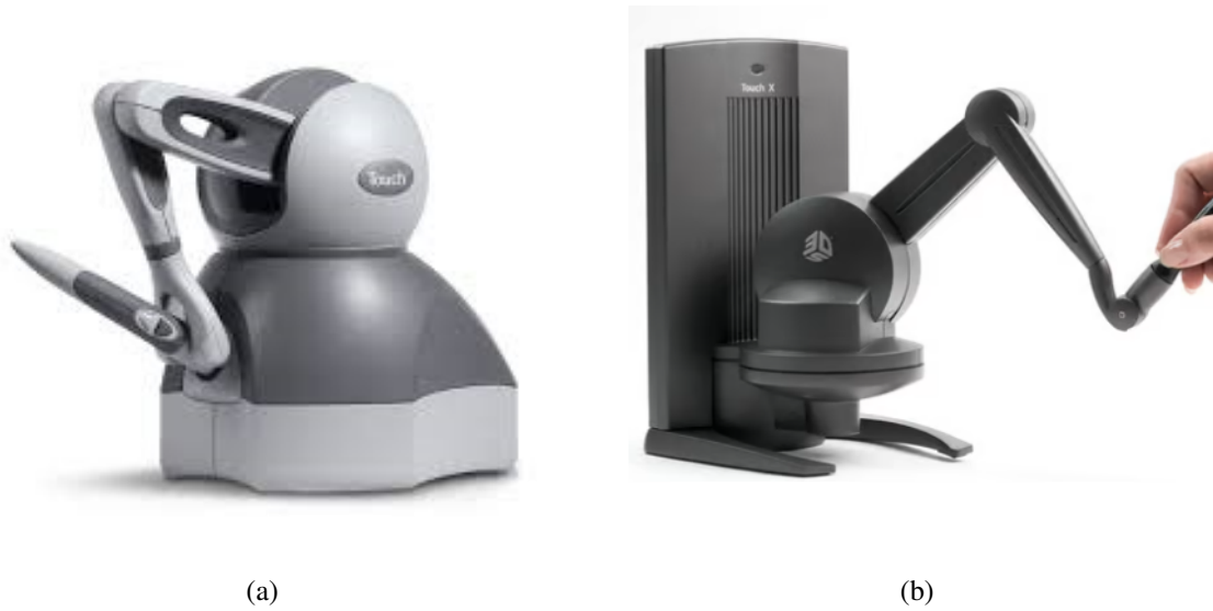
Figure 3.3: The teleoperation devices, touch and touch X.
