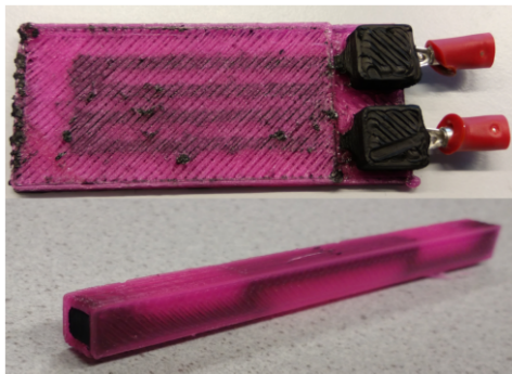
(a) 3D Printed Strain Sensors (Dijkshoorn et al. , 2018) (Creative Commons Attribution 4.0)
