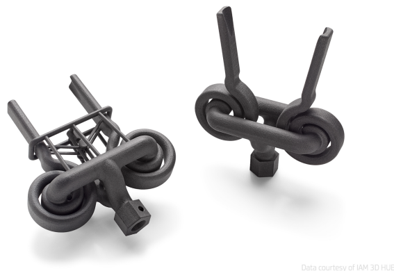
Figure 2.5.15: MJF Pneumatic Gripper (IAM 3D Hub, 2018). Image used with permission from IAM3DHub-Leitat.
