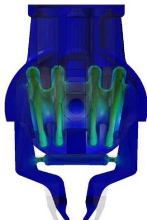
Figure 2.5.12: Integrated bellow gripper (Grzesiak et al. , 2011) ©Emerald Publishing Limited all rights reserved.
