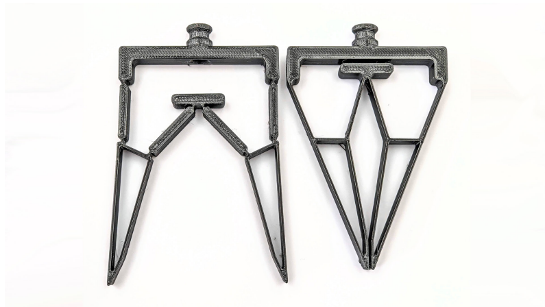
Figure 3.2.21: Plastic Deformation on Concentrated Compliant Gripper
