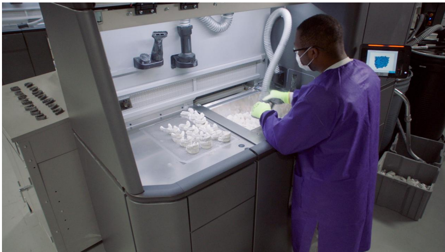
Figure 1.0.1: Multi-Jet Fusion Manual Part Extraction (Hartzell and Moore, 2019). Image used with permission from SmileDirectClub.
