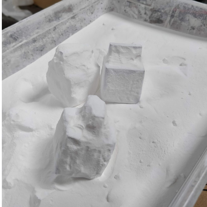
Figure 8.0.1: Caked Objects in Aged Powder from MJF Process
