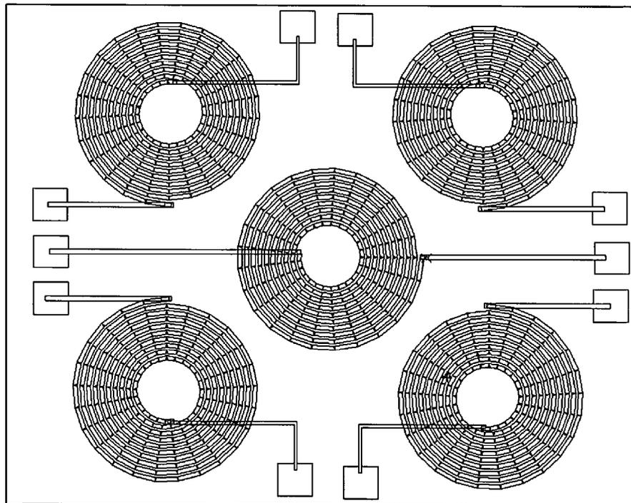
(57) Abstract: A magnetic particle detector system comprises a plurality of reaction surfaces; a corresponding plurality of electrical coils, each located adjacent a respective reaction surface; and a measuring system for measuring the effect of magnetic particles bound to a reaction surface on the inductance of the associated electrical coil.
