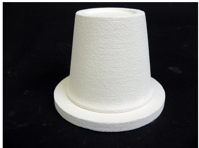
Figure 2 3D printed test cup on firing support
