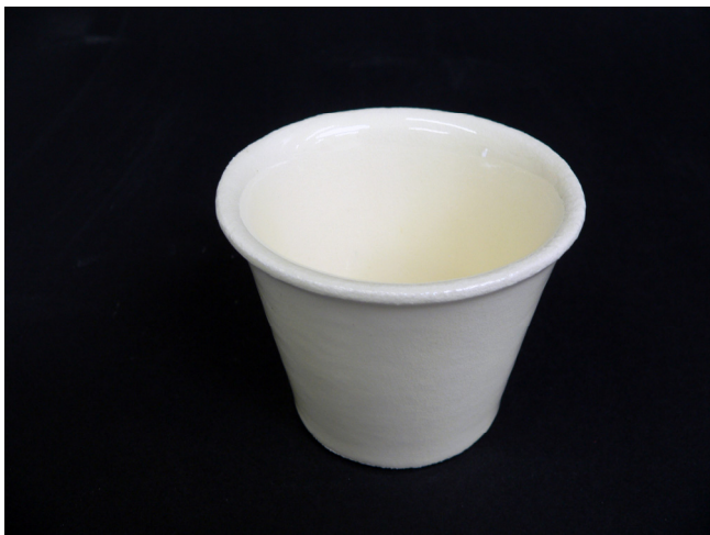
Figure 4 Fired glazed test cup
