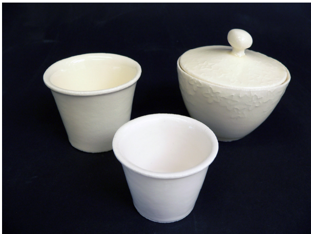
Figure 10 3D printed ceramic concept models
