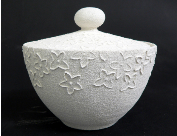
Figure 8 3D printed unfired ceramic sugar bowl and lid
