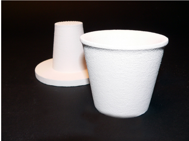
Figure 3 Test cup and firing support
