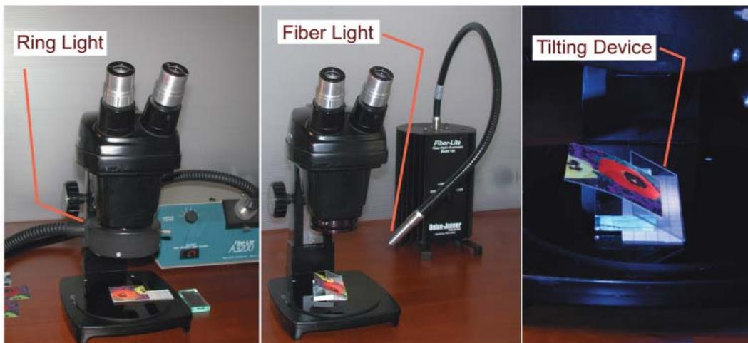
Fig. 2 Left: ring light mounted on the microscope provides uniform illumination. Centre: the self-supporting fibre provides illumination at variable angles for the tilted sample. Right: close-up of tilting device. The tilted slide is supported by a glass block. The bottom slide is covered with millimeter graph paper, providing a size reference.
