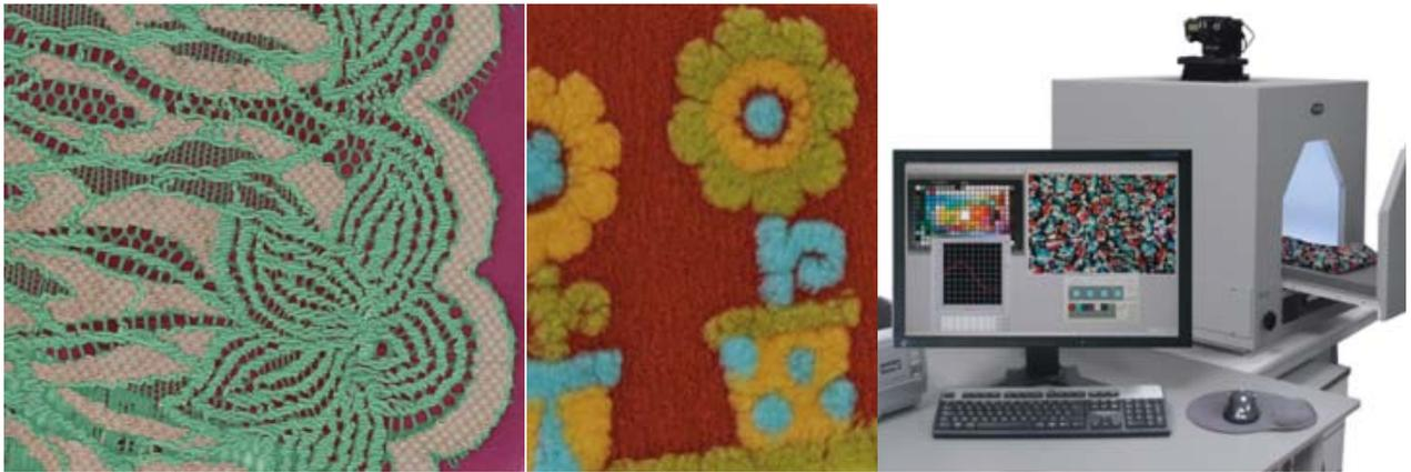
Fig. 9 Highly structured lace (left) and multicoloured pile fabric (middle) specimens which cannot be measured by conventional instruments. Photos courtesy VeriVide Ltd. ([www.verivide.com](http://www.verivide.com); [www.digieye.co.uk](http://www.digieye.co.uk))
