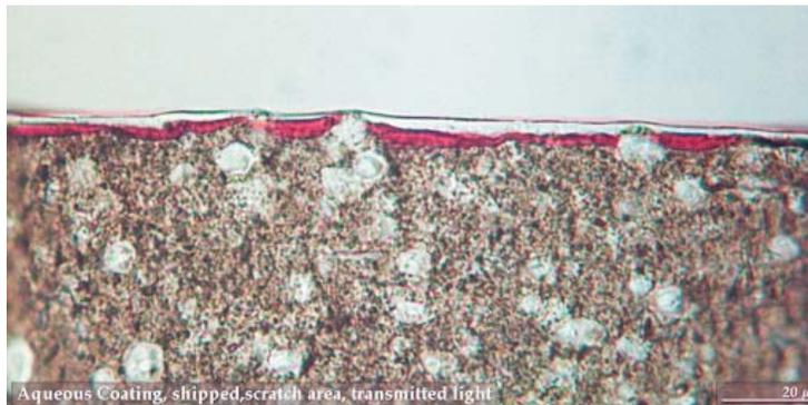
Fig. 11 The cross-section of the sheet shown in figure 10 shows large particles in the substrate that protrude from the surface and disrupt the ink layer and the shellac layer. These protrusions could scratch the surface of an adjacent coin holder during shipping.
