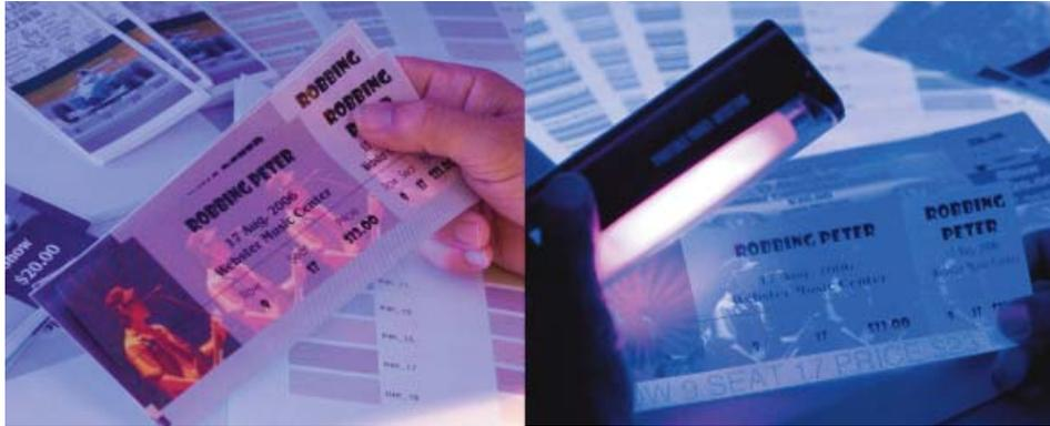
Fig. 3 A sample ticket under normal illumination (left) and under UV illumination (right) with the security text clearly visible.
