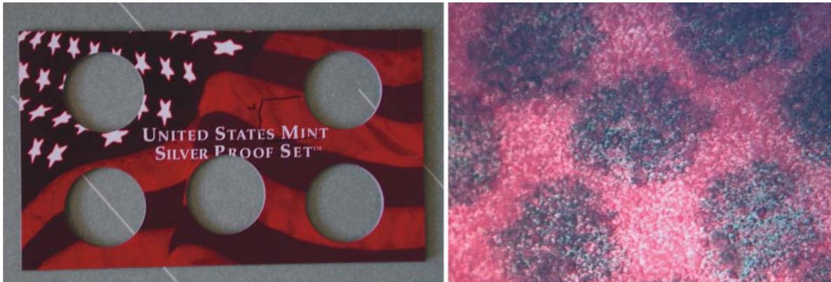
Fig. 9 Printed coin holder and surface view of original printed sheet, showing uniform optical density of print, and uniform texture on surface. Micrograph magnification is about 150X.
