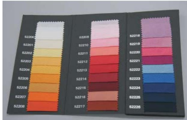
Fig. 3 Viscose fabric shade card with arbitrary sample coding. Samples are arranged according to hue and nuance.
