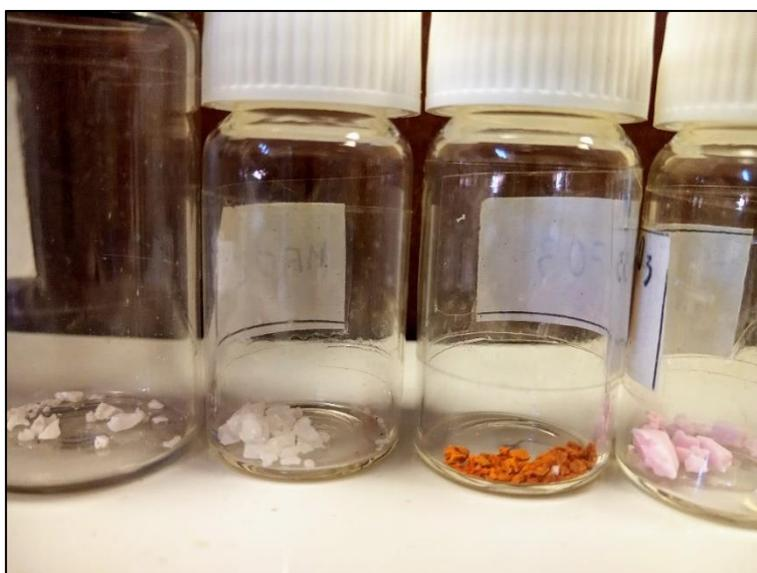
Fig. 4 The metal oxide nanopowder synthesised: from left to right  $\text{ZrO}_2\text{:Eu}^{3+}$ ,  $\text{ZrO}_2\text{:Y}^{3+}$ ,  $\text{ZrO}_2\text{:Tb}^{3+}$  and  $\text{ZrO}_2\text{:Er}^{3+}$
