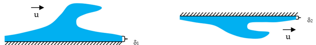
Figure 2. A schematic representation of liquid ‘roll wave’ and film thickness in a horizontal circular pipe: the bottom wave propagation (left) and up wave propagation (right). Parameter \delta represents the liquid film thickness and u is flow velocity.
