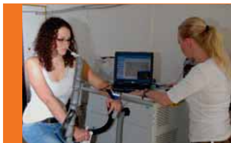
Figure 2. Photo of a SIFT mass spectrometer analysing VOCs in the breath of a volunteer in real time. Reproduced with kind permission of Patrik Španel.
