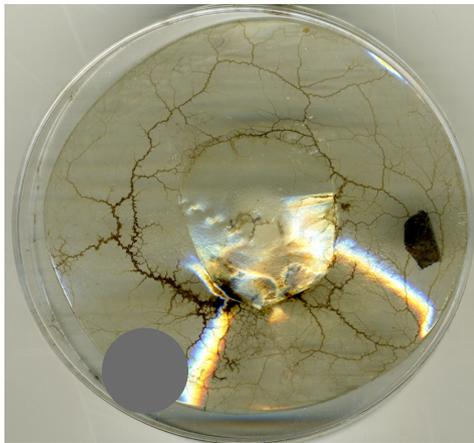
FIGURE 14. Towards *Physarum* wires. Control of magnetic nanoparticles in protoplasmic network. Position of 25×20 mm N52 neodymium magnet is shown by grey disc. Segments of the tubes closest to the magnet exhibit black colour indicating a high concentration of the internalised magnetic material.
