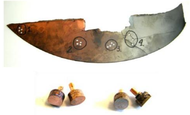
Fig. 5. Selection of the composite base material for the preparation of contact samples (1 ... 4 example of samples number of different chromium content)
