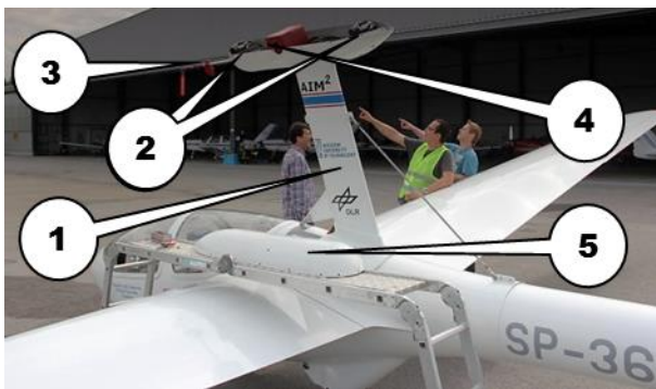
Figure 6 Dorsal camera pod installation on the PW-6U glider; (1) composite mast, (2) two IPCT cameras, (3) aerodynamic probe for pressure and \alpha - \beta -angle measurement, (4) one infrared thermography (IRT) camera, (5) disassembled housing cover
