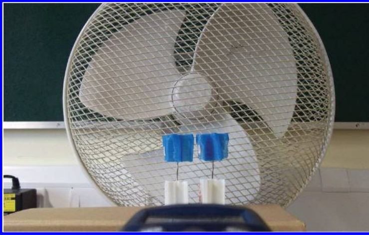
Figure 6: VAWT array experimental setup.
