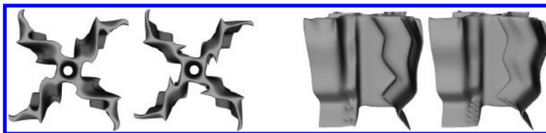
Figure 10: SCGA-ELS fittest evolved interacting VAWTs after 160 fabrications; 2692 rpm.
