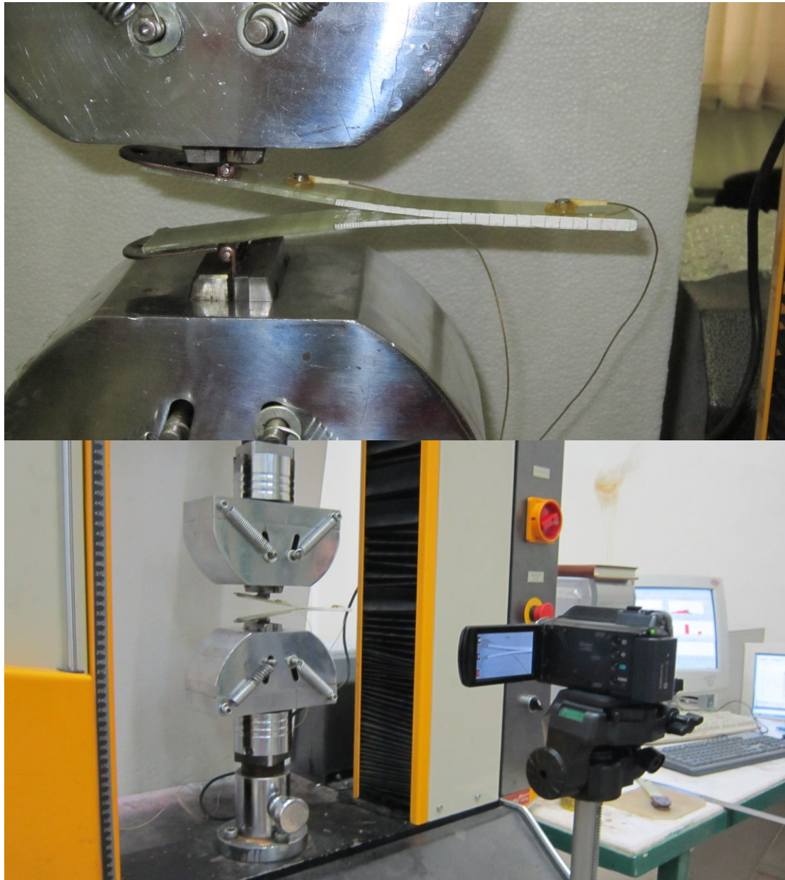
Fig. 2 Experimental setup for specimens loading and the AE apparatus
