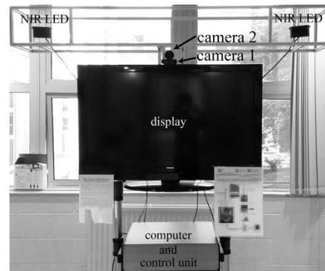
**Fig. 8.** System structure for the 2D+3D imaging system
