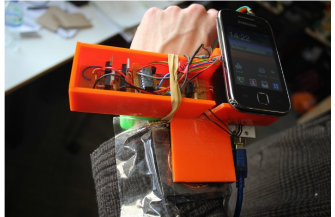
Fig. 13. Participant wearing the on-body garment power sharing distribution system, transferring power from the designated transmitter in the jacket pocket to the smartphone based on the wrist.
