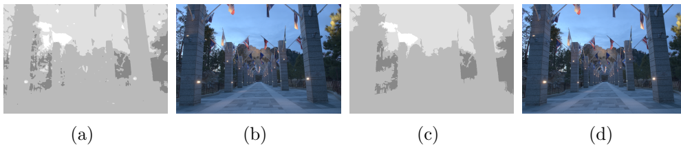
Figure 16: An example of differences between our GPU and CPU version of the algorithm on an image: (a) the zones map using our approximated algorithm on the GPU; (b) the tone mapped image using the GPU method; (c) the zones map using the original algorithm. Note that the red squares are the largest areas which differs from the GPU version; (d) the tone mapped image using the original algorithm.
