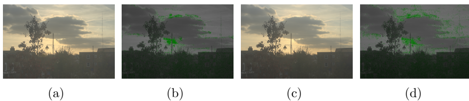
Figure 12: An example of DRIQAM [8] (note that green, blue and red respectively identify loss of visible contrast, amplification of invisible contrast and contrast reversal): (a) An image tone mapped using our method. (b) The amplification/loss/reversal map resulting after comparing (a) and the original HDR image. (c) The same image in (b) tone mapped with ATTM image tone mapped using our method. (d) The amplification/loss/reversal map resulting after comparing (c) and the original HDR image.
