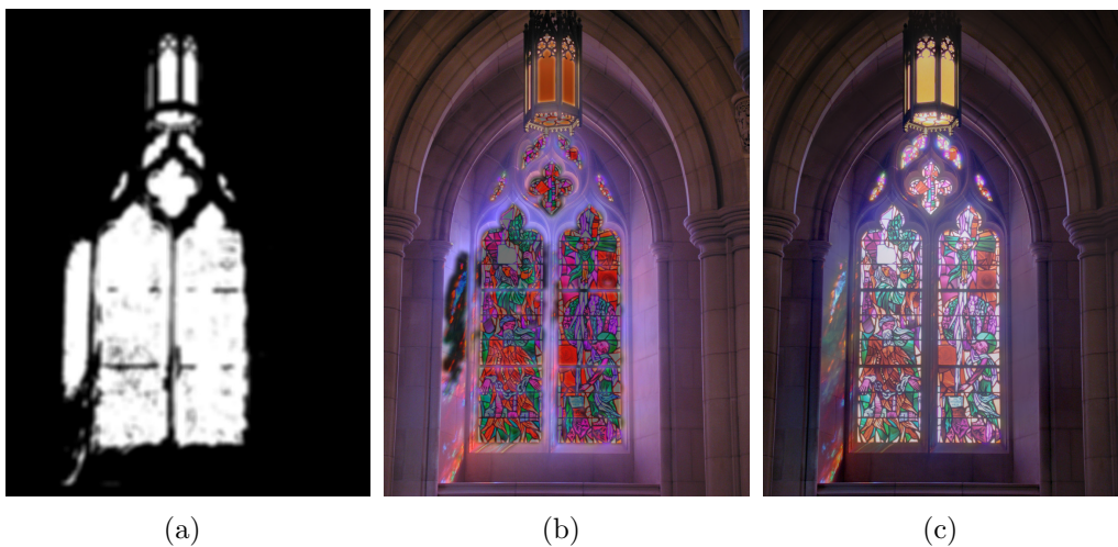
Figure 8: Comparison of the results obtained with two different fusion schemes: (a) the TMOs weight map; (b) a result using the simple fusion scheme; (c) a result using the proposed fusion scheme. Artifacts are visible on the image obtained with the simple fusion scheme (b). The original image is copyright of Max Lyons.
