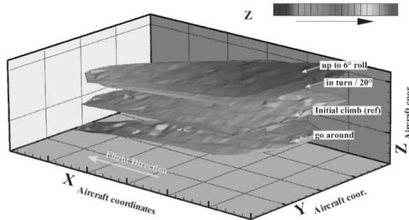
Figure 3. Wing tip displacement of a large airliner in different flight conditions
