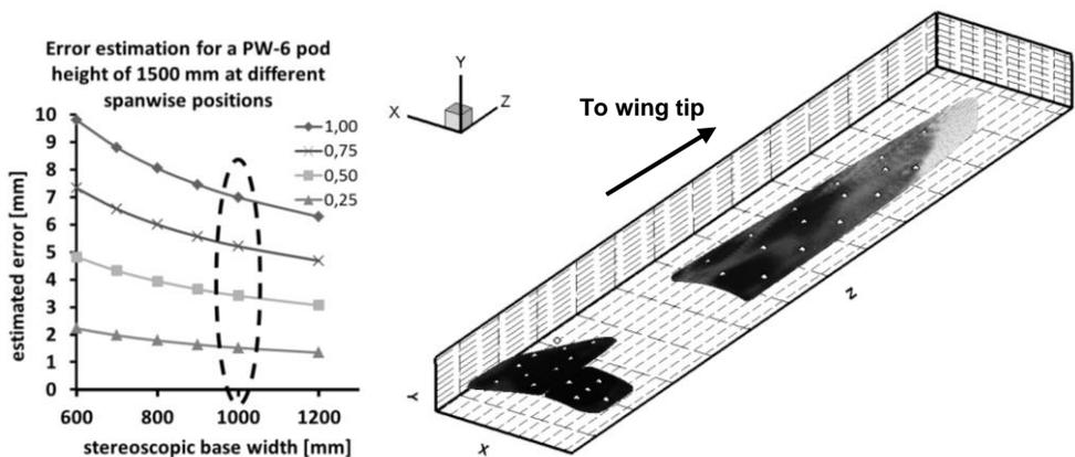
Figure 8. Theoretical error estimation in spanwise direction for different distances between two cameras (left); processed ground shape recording of the port wing overlaid with a greyscale code for standard deviation of 100 averaged IPCT image pairs; the darker the better (right)
