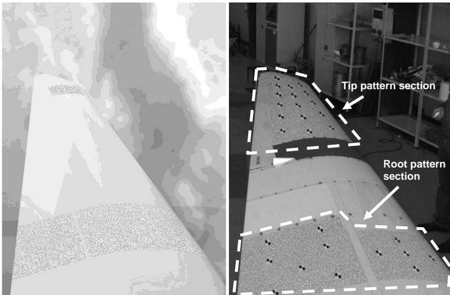
Figure 7. Comparison of virtual (left) and real (right) field of view of one IPCT camera
