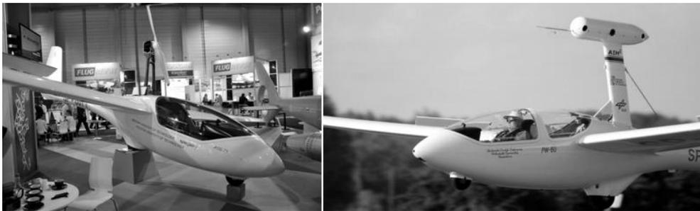
Figure 4. Electric glider AOS-71 (left) and finally used unpowered glider PW-6U with dorsal camera pod (right)
