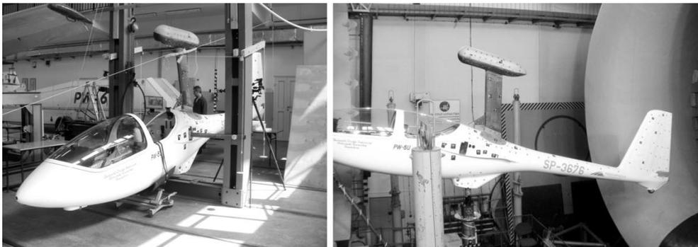
Figure 6. Static test (left) and wind tunnel test (right) performed to prove the stiffness, strength and stability of the camera pod
