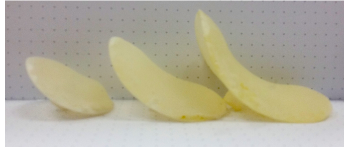
Fig. 14. Soft test pieces spread circumferentially around sensor, 60°, 90° and 120° left to right. Soft lumps are made from cast Platsil 7315 rubber silicone.
