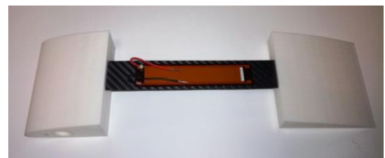
Figure 4. Manufactured and partially assembled wing with MFC actuator bonded on top of the smart composite rib.
