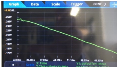
Fig.4. Measured liner terminal voltage drop with time demonstrated the Lithium battery has been stabilized after completion of the post-charge diffusion process
