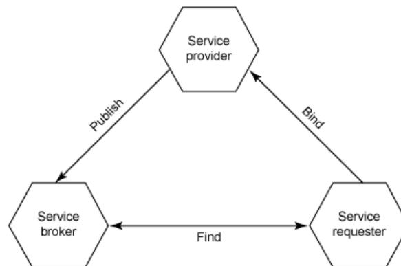
Figure 2.10: Service Oriented Architecture Model (Newcomer and Lomow, 2005)
