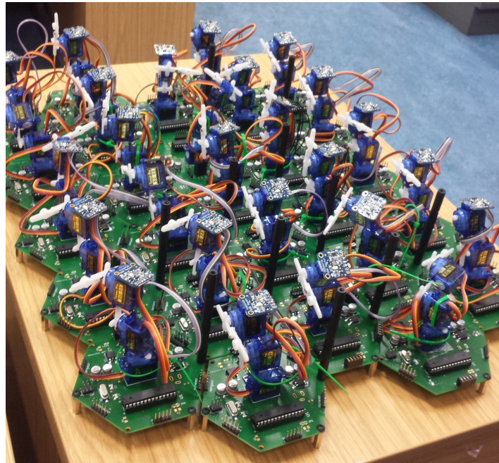
Figure 6. Multiple-tiled hexagonal cilia connected to each neighbour, sharing power and data.
