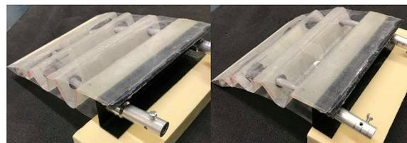
Fig. 5. Final camber morphing flap assembly.
