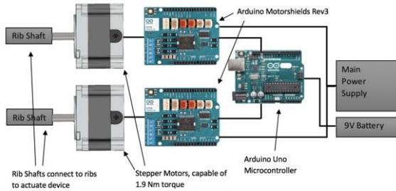
Fig.3. Visualisation of hardware setup for automating the morphing mechanism, showing the Arduino Uno (right) and two Arduino Motorshields Rev3, one for each motor (middle), connected to the wing ribs (left).
