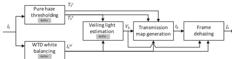
Fig. 2. Block diagram of the proposed approach. Temporal smoothing of the parameters takes place in each buffer. KEY –  $I_k$ : input frame at time  $k$ .  $T_k^b$ : Boolean value indicating whether pure haze regions exist;  $T_k^v$ : threshold value indicating amount of pure haze in frame;  $I_k^W$ : water-type dependent (WTD) white balancing output frame;  $V_k$ : veiling light estimate;  $t_k$ : transmission map;  $J_k$ : dehazed frame.
