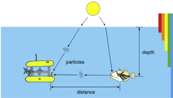
Fig. 1. Light is absorbed and scattered as it travels on its path from source, via objects in a scene, to an imaging system onboard an Autonomous Underwater Vehicle.
