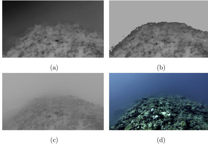
**Fig. 5.** Examples of transmission maps generated from the first frame from sequence  $S_4$  (Fig. 8 (a)). (a) Map estimated with green-blue dark channel (Drews-Jr et al., 2013). (b) Map with adapted transmission values. (c) Map refined with Laplacian image matting filter (Levin et al., 2008). (d) Output frame. (For interpretation of the references to colour in this figure legend, the reader is referred to the web version of this article.)
