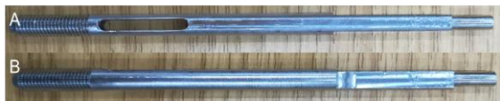
Figure 2 New orthopaedic for electromagnetic sensor. 2-A: front view with the anchoring system section and the cavity, 2-B: side view.
