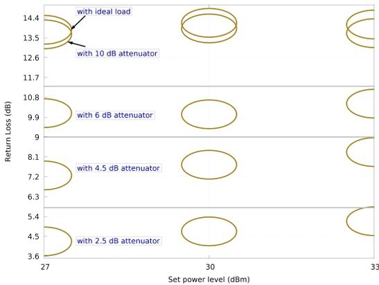
Fig. 19: Return loss with directional couplers in place to calibrate forward and reverse power
