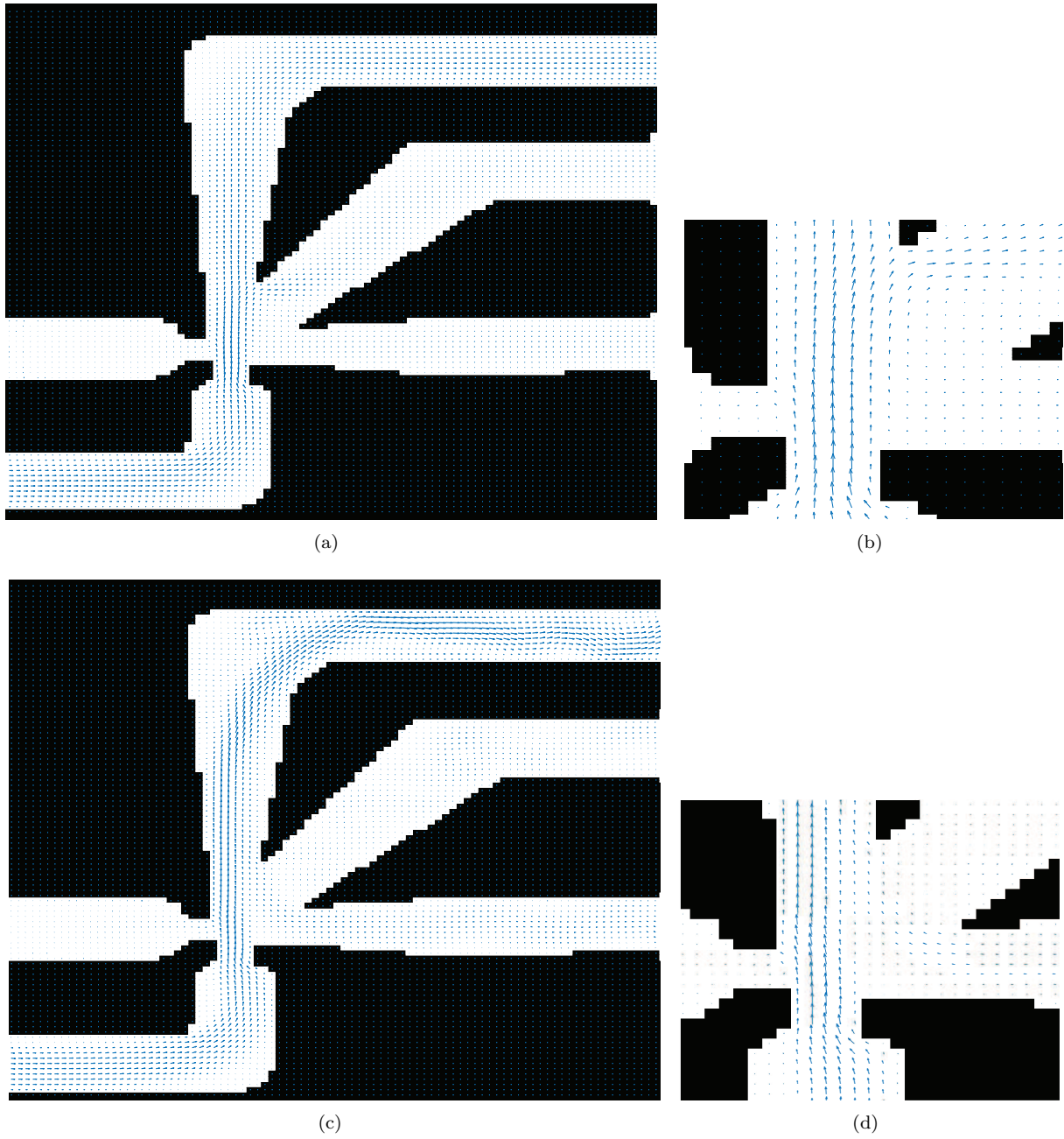
Figure 3: Flow field for AND gate (Fig. 2a) with input A activated for (ab) low, Re = 50 , and (cd) high, Re = 350 , Reynolds numbers. (ac) Overview of flow fields. (bd) Zoomed flow fields in the nozzle area.
