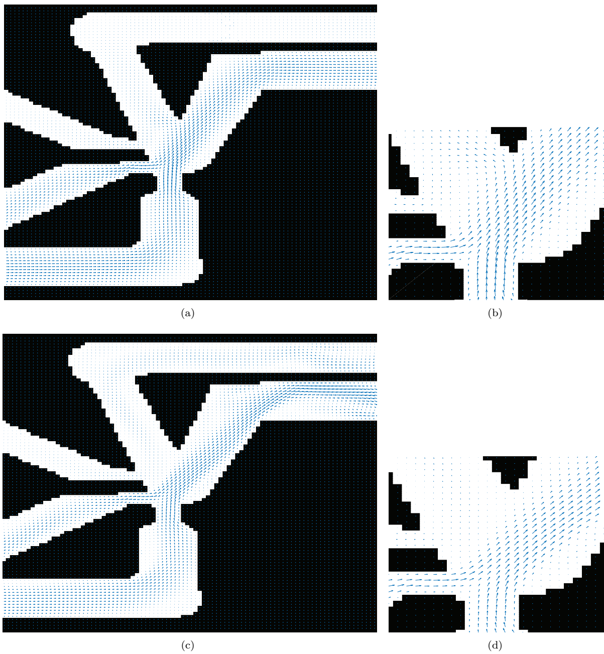
Figure 7: Flow field for OR gate (Fig. 2b) with input A activated for (ab) low, Re = 50 , and (cd) high, Re = 350 , Reynolds numbers. (ac) Overview of flow fields. (bd) Zoomed flow fields in the nozzle area.
