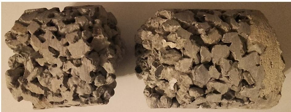
Fig 1. Sample of one of the NFC walls under study composed by 280mm NFC and 15mm thick external render
