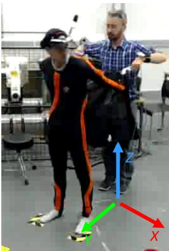
Fig. 3. Training data for this work was gathered from a human-human interaction study where 12 users were given assistance with putting on a jacket whilst wearing an Xsens motion tracking suit.
