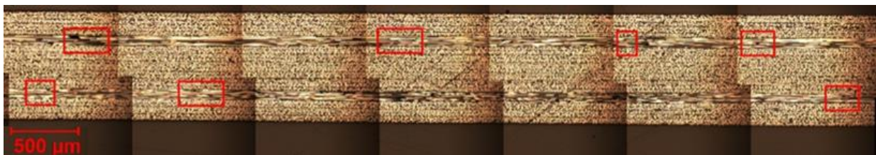
Figure 14: Microscopy for a AP-[ \pm 22.5_3/0_2/\pm 22.5_3 ] s specimen. The full width image is a mosaic at 10x magnification. Red rectangles highlight the locations of fragmentations.
