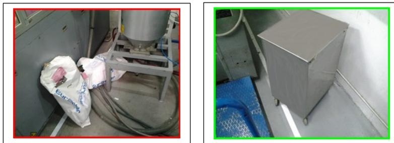
Figure 8. Inappropriate storage of the thermoplastic resin.
