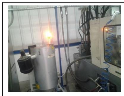
Figure 9. Implementation of poka-yoke: Sensor with alarm.
