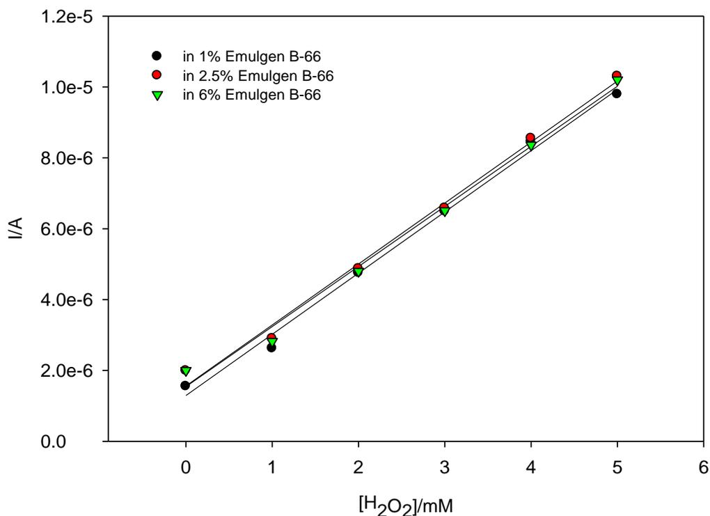
**Fig. 5.6. Chronoamperometric measurement of H<sub>2</sub>O<sub>2</sub> in 1, 2.5 and 6% (w/v) Emulgen B-66 (-0.1 V vs Ag/AgCl) in stirred batch solution.**
