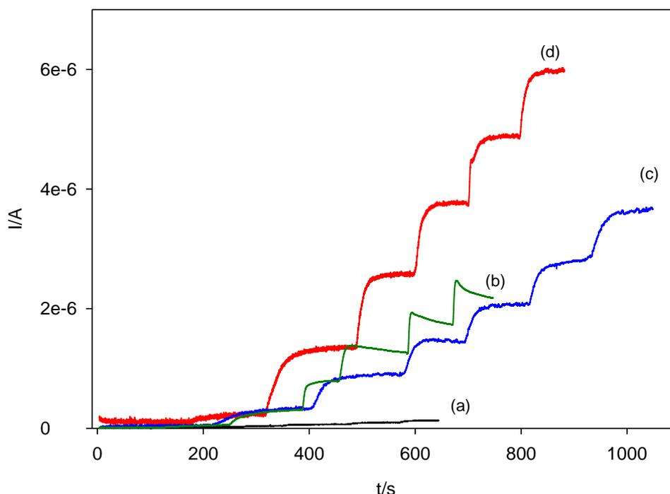
**Fig. 4.8. Amperometric measurement of 0.5 to 3 mM  $\text{H}_2\text{O}_2$  at  $-0.1$  V vs. Ag/AgCl in 5 ml stirred batch solution using: a) unmodified silver electrode in PBS; b) unmodified silver electrode in 6% (w/v) Emulgen B-66, c) modified electrode in PBS and d) modified electrode in 6% Emulgen B-66.**
