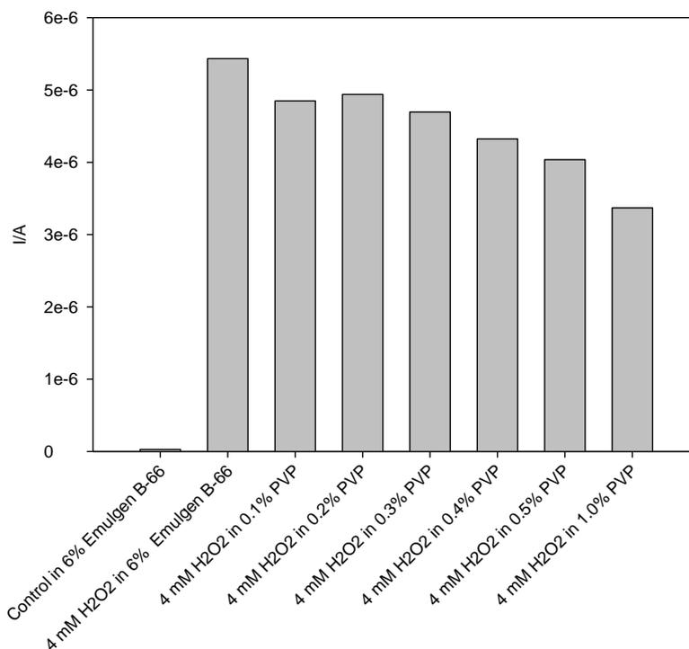
**Fig. 6.13. Effect of PVP concentration on chronoamperometric measurement (-0.1 V vs Ag/AgCl) of 4 mM H<sub>2</sub>O<sub>2</sub> in the presence of different concentrations of PVP using modified electrodes in non-stirred batch solution, delipidated serum was used for control experiments.**
