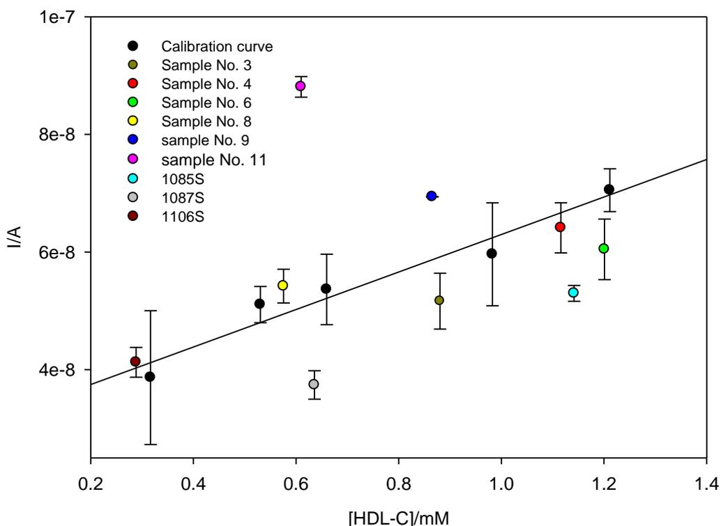
**Fig. 5.23. Amperometric responses of the HDL-C biosensor to clinical serum samples.**
