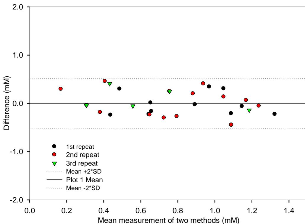
**Fig. 5.25. Bland–Altman plot of the difference between sensor/abcam assay kit against the mean measurement of two methods in the 26 measurements**
