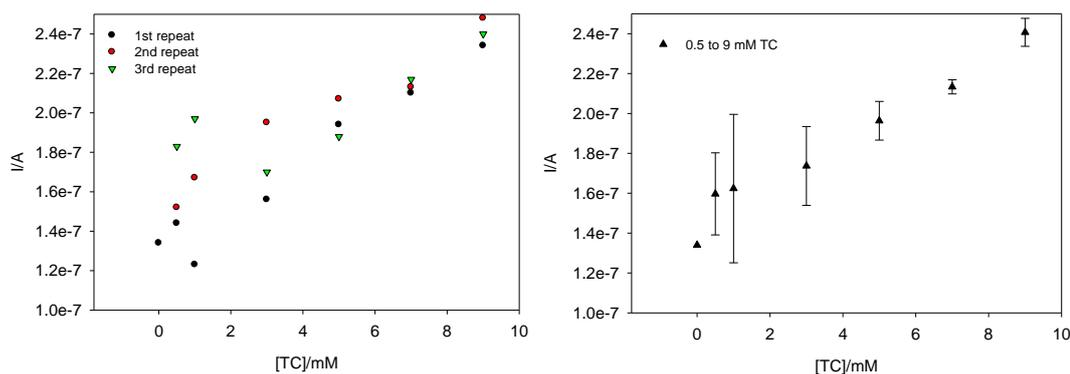
**Fig. 6.25. Measurement of TC using unmodified silver paste electrodes (slope= $9.38 \times 10^{-9}$  A/mM and  $r^2$  of 0.982, RSD=9.5%; n=3).**
