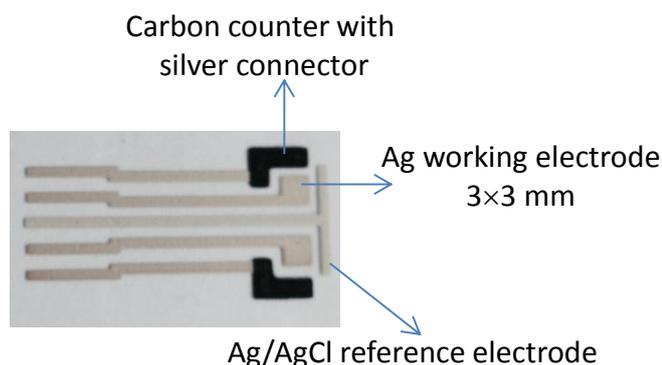
**Fig. 2.1. Image of the dual electrode system fabricated using screen printing.**
