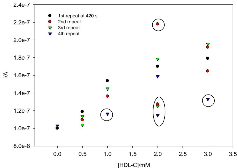
**Fig. 6.4. Chronoamperometric measurement (-0.1 V vs Ag/AgCl) of HDL-C using encapsulated HDL-C biosensors using 10 layers of inkjet-printed assay reagent deposited on both silver electrodes, after 240 s incubation at room temperature, (slope= $2.42 \times 10^{-8}$  A/mM,  $r^2=0.958$ ).**
