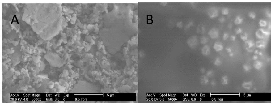
**Fig. 6.1. SEM images of modified electrodes: A before drop-coating of assay reagent and B after deposition. Acceleration voltage of 20 keV. (5000x magnification). using GSE detector.**
