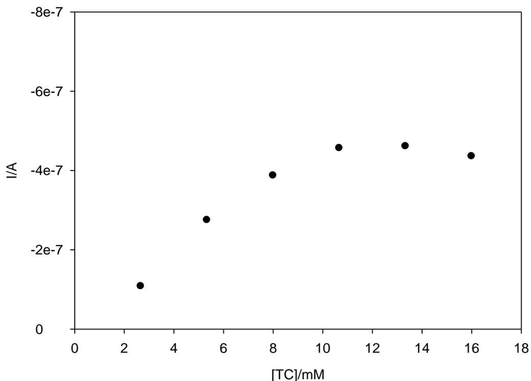
**Fig. 5.26. Amperometric response of the TC biosensor at 420 s to 2 to 16 mM TC in the presence of 23 U/mL ChOx, 39 U/mL ChEs and 0.5% (v/v) Triton X-100 (240 s incubation time was applied)**
