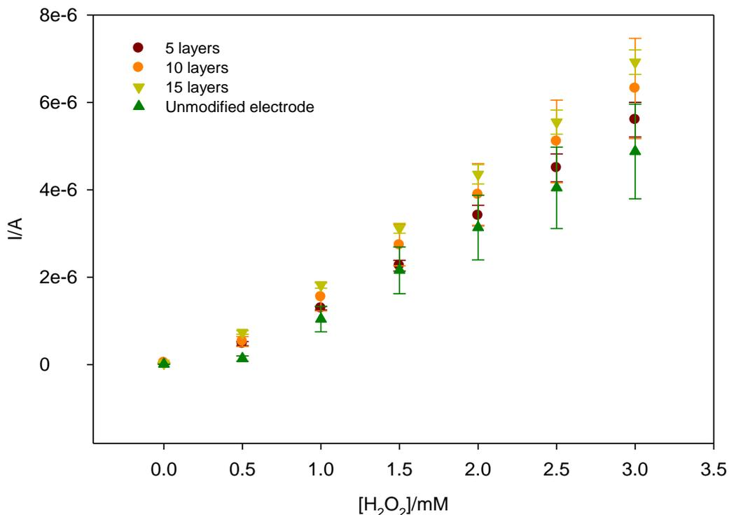
**Fig. 5.18. Amperometric measurement of 0 to 3 mM H<sub>2</sub>O<sub>2</sub> in 6% (w/v) Emulgen B-66 using 0, 5, 10 and 15 layers inkjet-printed 6% (w/v) Emulgen B-66/PBS modified electrodes (n=3) (stirred batch experiment).**
