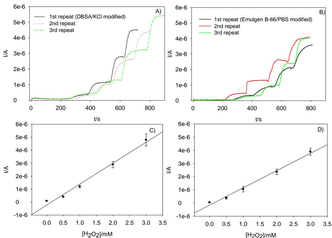
**Fig. 5.19. Comparison of electrode response to  $H_2O_2$  with modification using DBSA/KCl or Emulgen-B66/PBS: A) DBSA/KCl modified electrodes and B) Emulgen B-66/PBS modified electrodes; Amperometric response to  $H_2O_2$  using: C) DBSA/KCl modified electrodes (Slope= $1.61 \times 10^{-6} A/mM$ ;  $r^2=0.988$ ) and D) Emulgen B-66/PBS modified electrodes (slope= $1.31 \times 10^{-6} A/mM$ ;  $r^2=0.991$ ). - 0.1 V vs. Ag/AgCl.**
