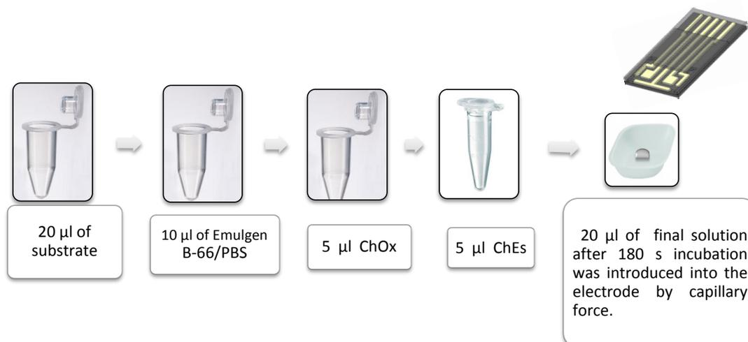
**Fig. 2.5. Schematic of assay reagent addition for amperometric measurement of HDL-C using external addition of reagents.**
