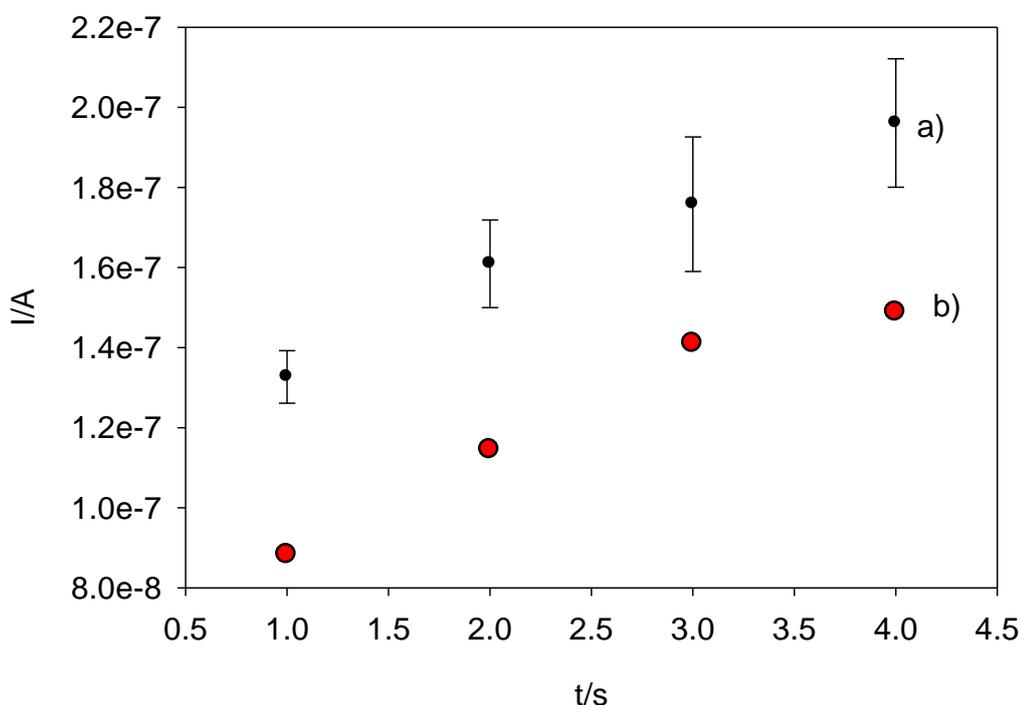
**Fig. 6.8. Chronoamperometric measurement of HDL-C using encapsulated HDL-C biosensors inkjet-printed using one layer of assay reagent  $15 \times 8$  mm<sup>2</sup> electrode surface after 240 s incubation at room temperature: a) 3 sets performed after printing (slope:  $2.05 \times 10^{-8}$  A/mM,  $r^2=0.984$ ,  $n=3$ ), b) set 4 performed 5 hrs after printing (slope:  $2.08 \times 10^{-8}$  A/mM,  $r^2=0.954$ ).**
