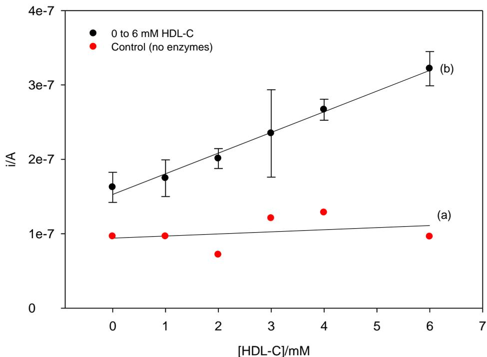
**Fig. 5.3. Biosensor response to 0-6 mM HDL-C in PBS at -0.1 V (vs Ag/AgCl). a) 0 mM in the presence of ChEs and ChOx and 1 to 6 mM in the absence of enzymes; b) in the presence of 1% (w/v) Emulgen B-66, 39 U/mL ChEs and 23 U/mL ChOx; (slope= $2.78 \times 10^{-8}$  A/mM,  $r^2=0.99$ ).**
