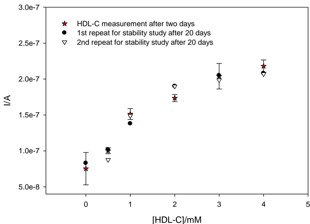
**Fig. 6.17. Amperometric measurement of HDL-C at -0.1 V vs Ag/AgCl using integrated biosensors with four printed reagent layers following: a) two and; b) 20 days storage at 2-8 °C. a) slope= $3.52 \times 10^{-8}$  and  $r^2=0.92$ ,  $n=4$ . b) slope= $3.33 \times 10^{-8}$  and  $r^2=0.87$ ,  $n=2$ .**
