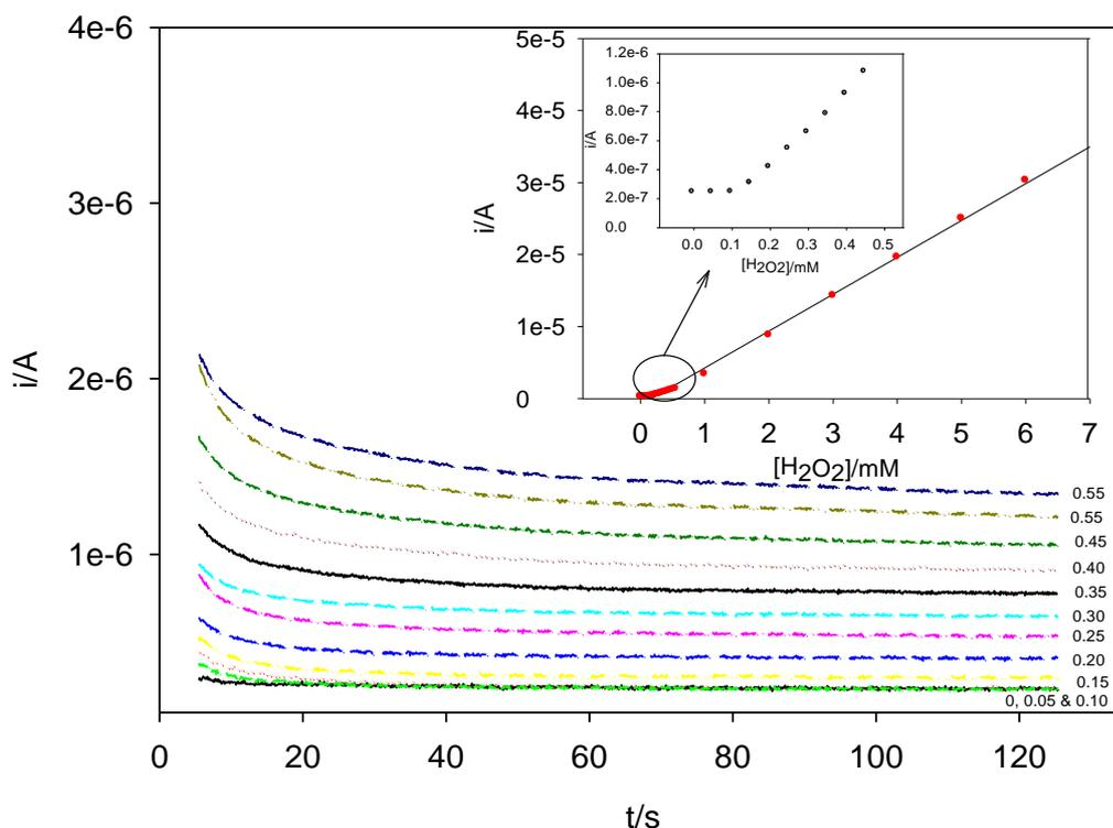
**Fig. 4.6. Chronoamperometric measurement of H<sub>2</sub>O<sub>2</sub> (0-0.55 mM) at modified electrodes in 0.1 M PBS pH 6.8, 1% (w/v) Emulgen B-66 at -0.1 V vs. Ag/AgCl. Inset: Current response at 120 s.**
