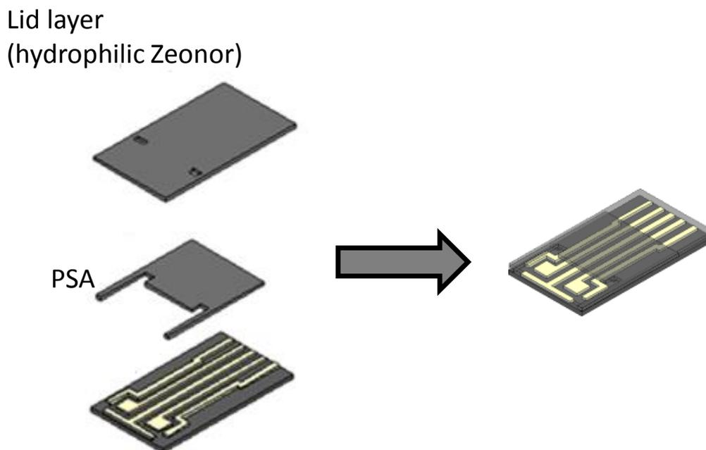
**Fig. 2.2. Design layout of the encapsulated electrodes**
