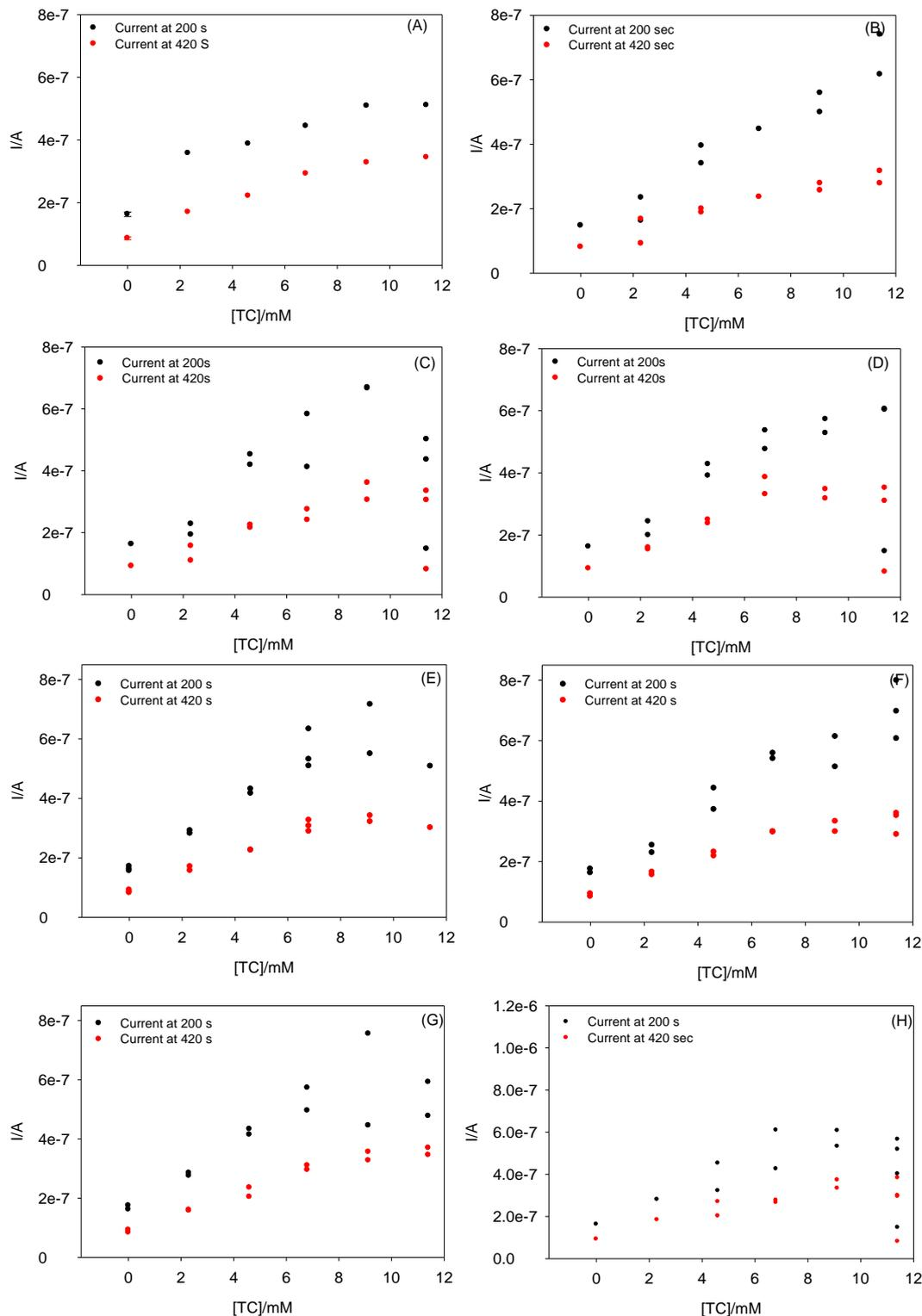
**Fig. 5.27. Amperometric response of the TC biosensor at TC concentrations of 0 to 11 mM at  $t=200$  s and 420 s in the presence of different ChEs/ChOx combinations: A) 78/20, B) 78/40, C) 78/60, D) 78/100, E)156/20, F) 156/40, G) 156/60 and H) 156/100 U/mL.**
