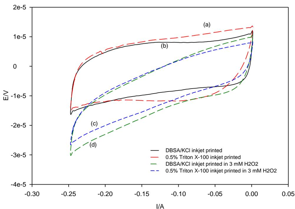
**Fig. 5.29. Cyclic voltammograms of electrodes modified in Triton X-100/PBS solution (a and c) or DBSA/KCl (b and d), measured in Triton/PBS (a and b) or Triton/PBS and 3 mM H<sub>2</sub>O<sub>2</sub> (c and d) (vs. Ag/AgCl).**
