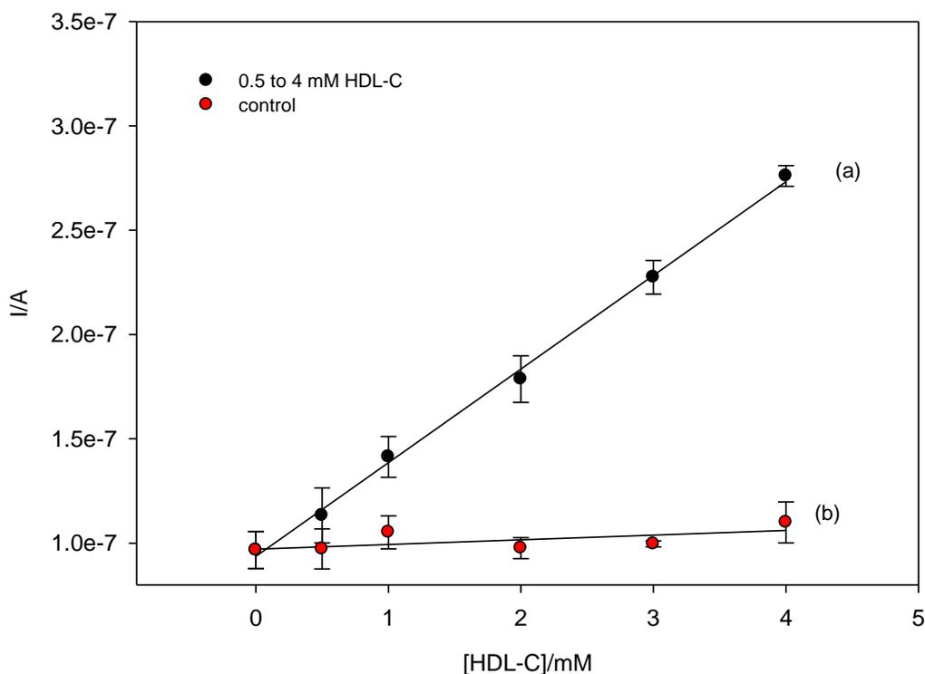
**Fig. 5.9. Biosensor response to HDL-C in delipidated serum at -0.1 V (vs Ag/AgCl); a) Biosensor containing 6% (v/v) Emulgen B-66, 39 U/mL ChEs and 23 U/mL ChOx; (slope= $4.49 \times 10^{-8}$ ,  $r^2=0.998$ ,  $n=3$ ) (240 s incubation time, due to 1 min for equilibrium); b) Biosensor controls in the absence of ChEs and ChOx (0.5 to 4 mM HDL-C) and in the presence of all assay components at 0 mM (delipidated serum).**
