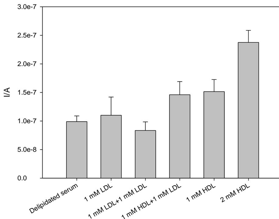
**Fig. 6.7. Chronoamperometric measurement (-0.1 V vs Ag/AgCl) of LDL-C, HDL-C and combination of HDL-C and LDI-C using using two layers of assay reagent inkjet-printed on 15 × 8 mm of Emulgen/PBS modified electrode, after 240 s incubation at room temperature (t=420 s).**
