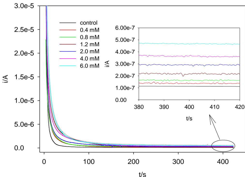
**Fig. 5.1. Chronoamperometric measurement of H<sub>2</sub>O<sub>2</sub> (0-6 mM) using encapsulated electrodes in the presence of HDL-C assay reagent at -0.1 V vs Ag/AgCl).**
