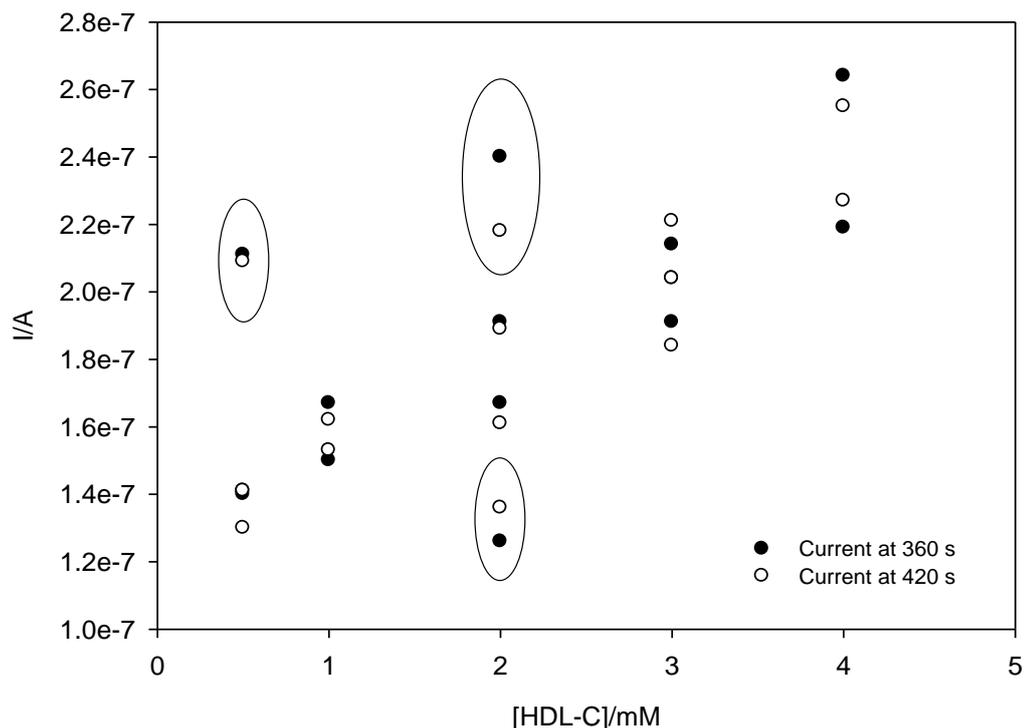
**Fig. 6.2. Chronoamperometric measurement (-0.1 V vs Ag/AgCl) of HDL-C using encapsulated HDL-C biosensors prepared using 10 layers of assay reagent inkjet-printed on Emulgen/PBS modified silver electrodes. The current was measured at 420 s after 240 s incubation; (slope= $1.76 \times 10^{-8}$  A/mM,  $r^2=0.745$ ).**
