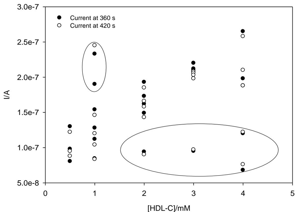
**Fig. 6.3. Chronoamperometric measurement (-0.1 V vs Ag/AgCl) of HDL-C using encapsulated HDL-C biosensors using 20 layers of inkjet-printed assay reagent deposited on a single Emulgen b-66/PBS modified silver electrode, after 240 s incubation at room temperature, (slope= $1.86 \times 10^{-8}$  A/mM,  $r^2=0.782$ ).**
