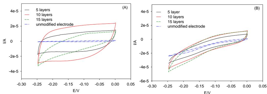
**Fig. 5.17. Cyclic voltammogram of 0, 5, 10 and 15 layers inkjet-printed 6% (w/v) Emulgen B-66 modified silver electrodes in A) 6% (w/v) Emulgen B-66/PBS and B) 3 mM H<sub>2</sub>O<sub>2</sub> prepared in 6% (w/v) Emulgen B-66/PBS solutions.**
