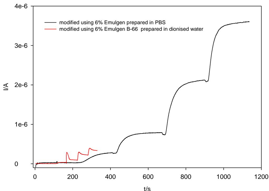
**Fig. 5.13. Amperometric measurement of 0 to 3 mM  $\text{H}_2\text{O}_2$  using modification solution containing: a) 6% (w/v) Emulgen B-66 prepared in deionised water and b) 6% (w/v) Emulgen B-66 prepared using 0.1 M PBS.**
