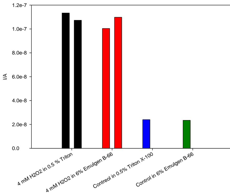
**Fig. 4.11. Chronoamperometric response to 8  $\mu$ L of 4 mM H<sub>2</sub>O<sub>2</sub> (-0.1 V vs Ag/AgCl) in the presence of 0.5% (v/v) Triton X-100 and 6% (w/v) Emulgen B-66 at 420 s. Delipidated serum was used for controls.**
