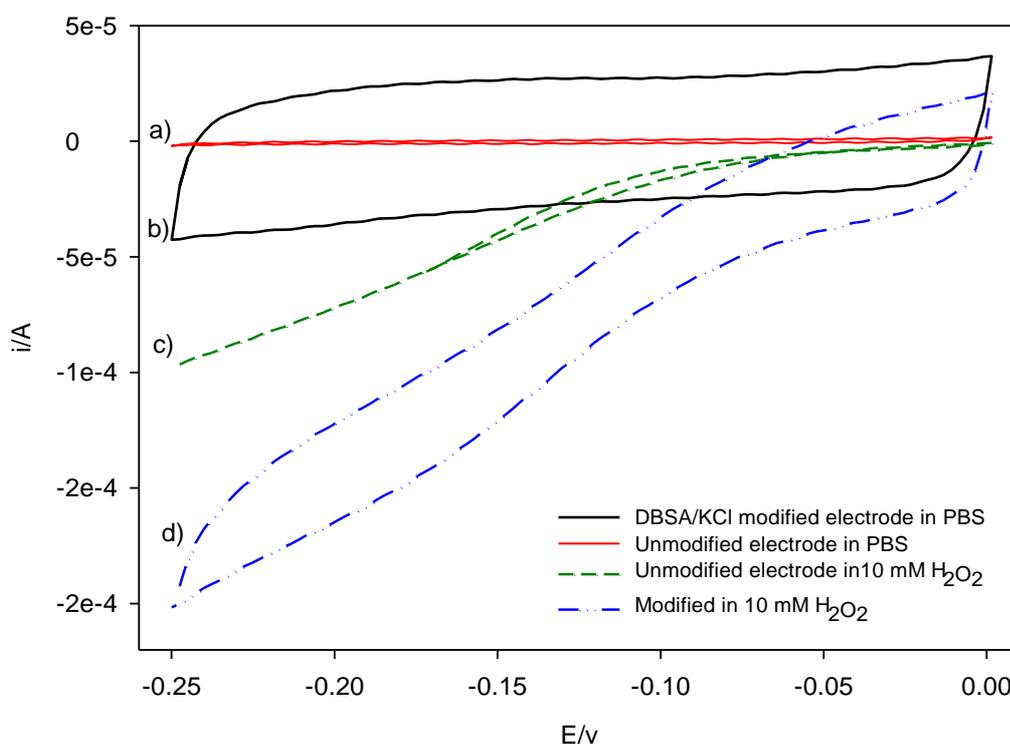
**Fig. 4.1. Cyclic voltammograms of silver electrodes measured in PBS and 10 mM H<sub>2</sub>O<sub>2</sub> (-0.25 to 0 to -0.25 V at 100 mV/s vs. Ag/AgCl): a) unmodified in PBS, b) modified in PBS, c) unmodified in 10 mM H<sub>2</sub>O<sub>2</sub>, d) modified in 10 mM H<sub>2</sub>O<sub>2</sub>.**
