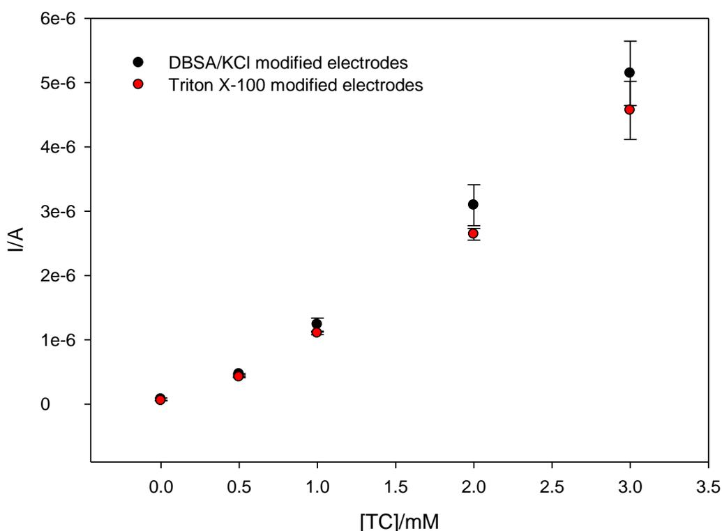
**Fig. 5.31. Amperometric response of electrodes modified using DBSA/KCl or Triton/PBS to  $\text{H}_2\text{O}_2$  in stirred batch solution at -0.1 V (vs. Ag/AgCl) (n=3).**
