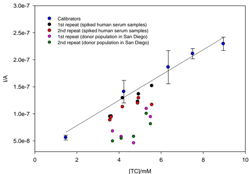
**Fig. 5.35.** TC biosensor responses to clinical samples at -0.1 V vs. AgAgCl, 420 s after 240 s incubation at room temperature, TC concentrations of 1.47, 4.23, 6.34, 7.50 and 8.96 were used as calibrators while the remaining were used for sample measurement which were either duplicate measurements of spiked human serum samples or the San Diego donor population.
