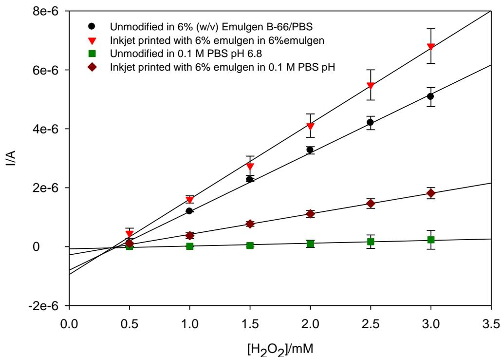
**Fig. 5.16. Amperometric response of un-modified electrodes and those modified using inkjet-printed of 6% Emulgen B-66/PBS to 0 to 3 mM H<sub>2</sub>O<sub>2</sub> in both PBS and 6% Emulgen B-66/PBS (stirred batch experiment).**
