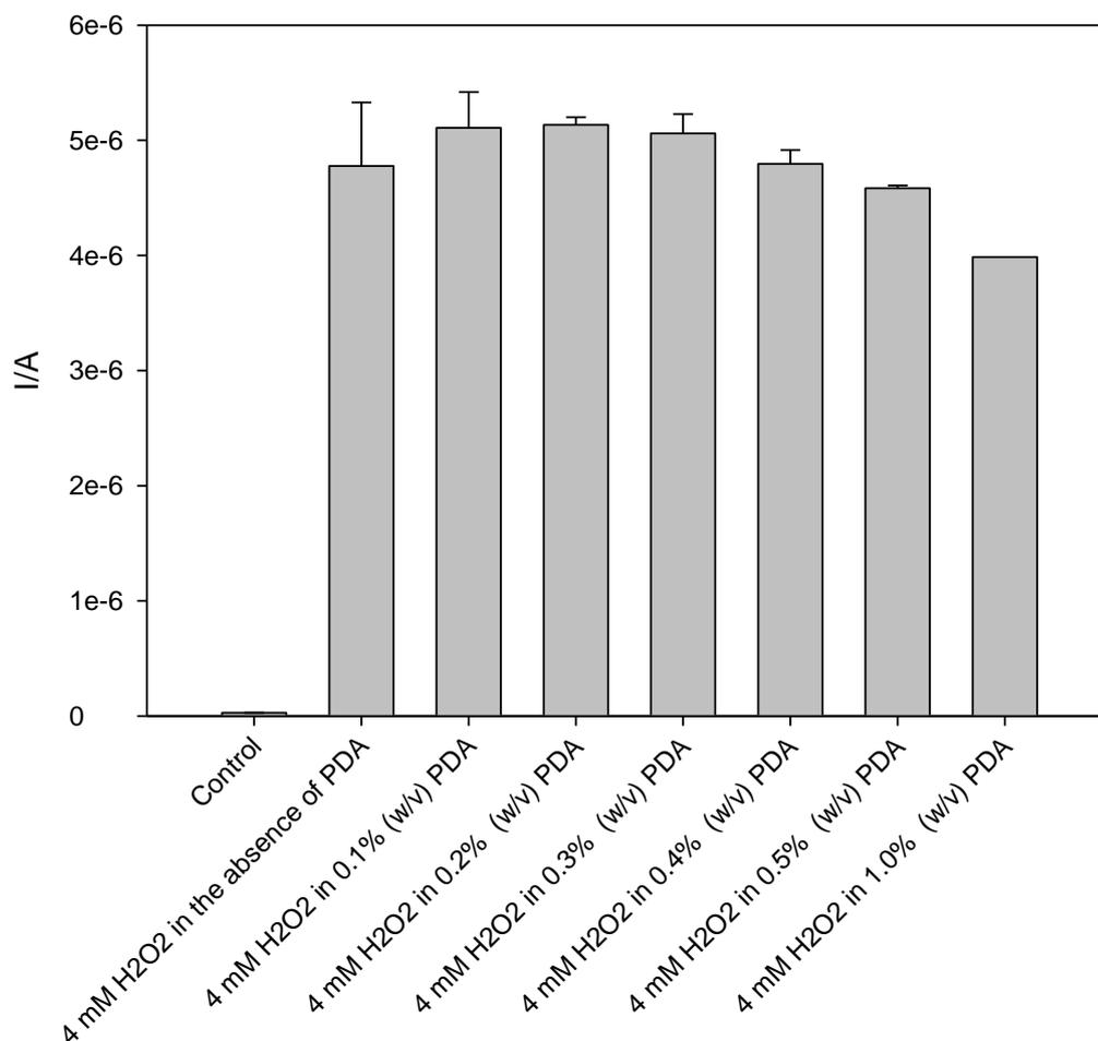
**Fig. 6.11. Effect of PDA concentration on chronoamperometric measurement (-0.1 V vs Ag/AgCl) of 4 mM H<sub>2</sub>O<sub>2</sub> in the presence of different concentrations of PDA using modified electrodes in non-stirred batch solution, delipidated serum was used for control experiments.**
