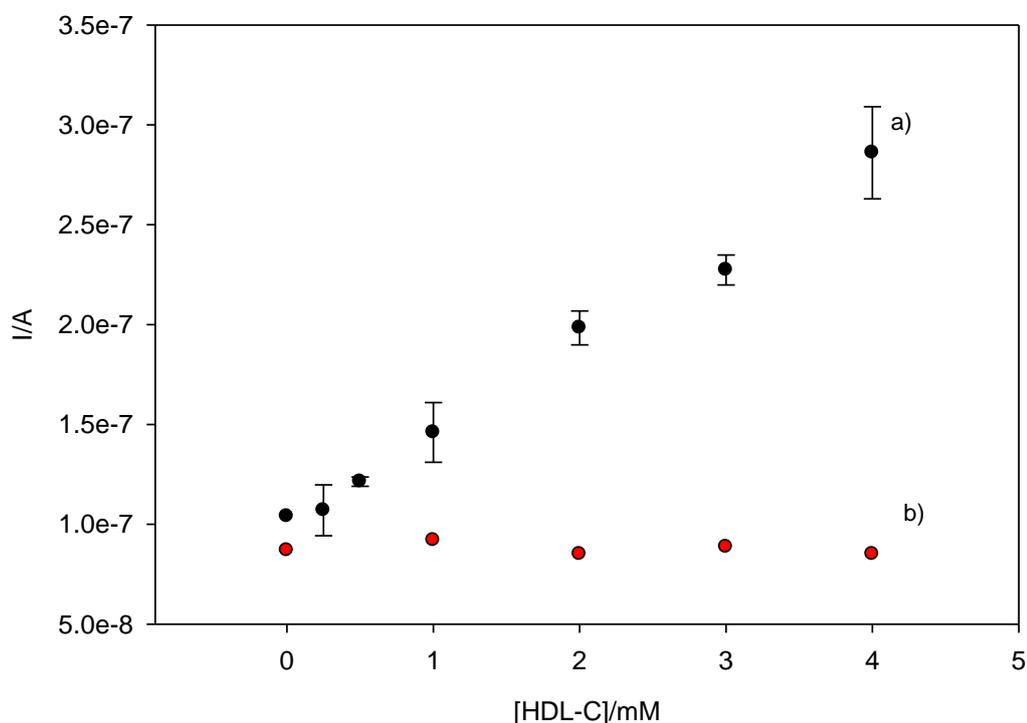
**Fig. 6.20.** a) Measurement of HDL-C using unmodified silver paste electrodes (slope= $4.55 \times 10^{-8}$ ,  $r^2=0.993$ , RSD=6.6%; n=3); b) control in the absence of enzymes.
