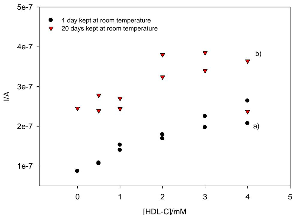
**Fig. 6.18. Amperometric measurement of HDL-C at -0.1 V vs Ag/AgCl using integrated biosensors with four printed reagent layers following: a) one (slop= $3.47 \times 10^{-8}$ ,  $r^2=0.95$ ,  $n=2$ ) and; b) 20 days storage at room temperature.**
