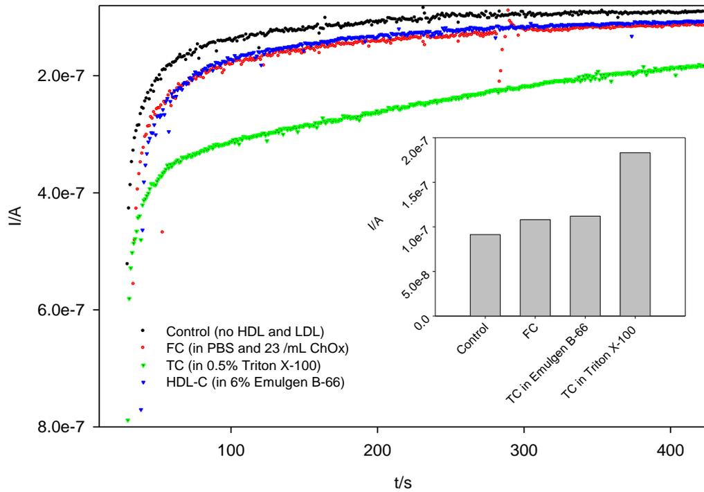
**Fig. 5.10. Chronoamperometric measurement of TC, HDL-C and FC present in delipidated serum containing 4 mM LDL-C using the developed biosensor. Inset: Biosensor response at 420 s in delipidated serum was used as control.**
