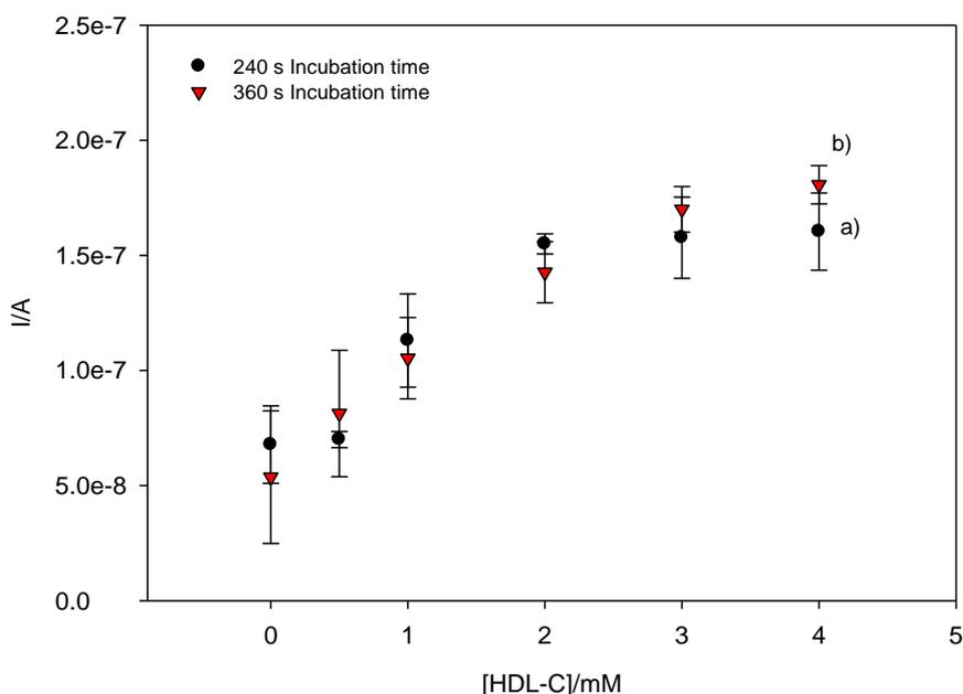
**Fig. 6.15. Amperometric measurement (-0.1 V vs Ag/AgCl) of HDL-C in delipidated serum using the integrated biosensor: a) after 240 s incubation (slope= $2.57 \times 10^{-8}$  A/mM and  $r^2 = 0.825$ ,  $n=3$ ) and b) after 360 s Incubation (slope= $3.20 \times 10^{-8}$  A/mM and  $r^2 = 0.952$ ,  $n=3$ ).**
