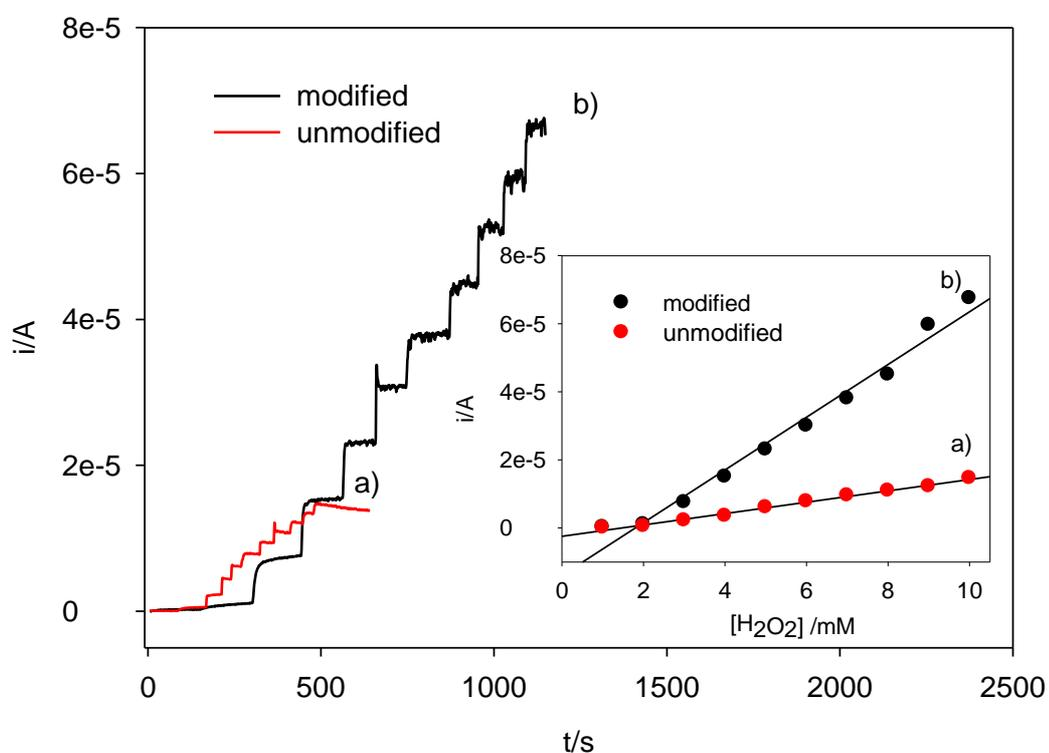
**Fig. 4.2. Amperometric responses of silver paste electrodes at -0.1 V (vs Ag/AgCl) in 0 to 10 mM  $\text{H}_2\text{O}_2$  in stirred batch solution: (a) unmodified and (b) modified, Inset: Plot of cathodic current vs the concentration of  $\text{H}_2\text{O}_2$  at -0.1 V (vs Ag/AgCl) a) modified (slope= $7.75 \times 10^{-6}$ ,  $r^2=0.98$ ), b) unmodified (slope= $1.67 \times 10^{-6}$ ,  $r^2=0.99$ ).**
