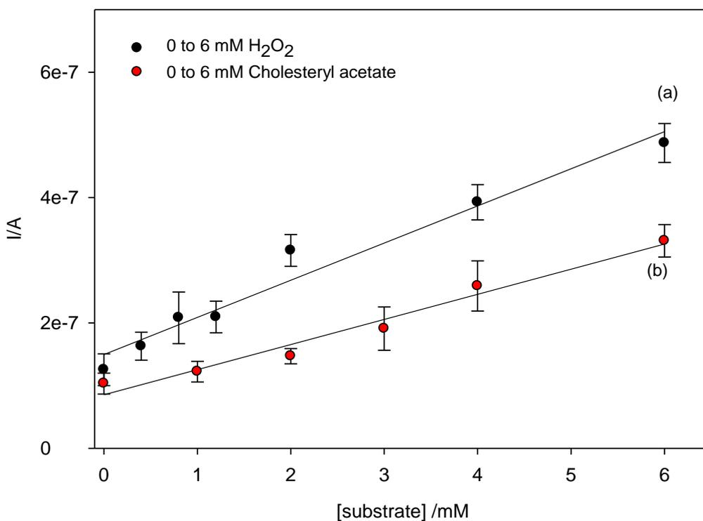
**Fig. 5.2. Chronoamperometric response to 8  $\mu$ L of (a) 0 to 6 mM H<sub>2</sub>O<sub>2</sub> and (b) 0 to 6 mM cholesteryl acetate (-0.1 V vs Ag/AgCl at 420 s) in the presence of HDL-C assay reagents at 420 s, (slope= $5.93 \times 10^{-8}$  A/mM,  $r^2=0.97$  for H<sub>2</sub>O<sub>2</sub> and slope= $4.01 \times 10^{-8}$  A/mM,  $r^2=0.97$  for cholesteryl acetate).**
