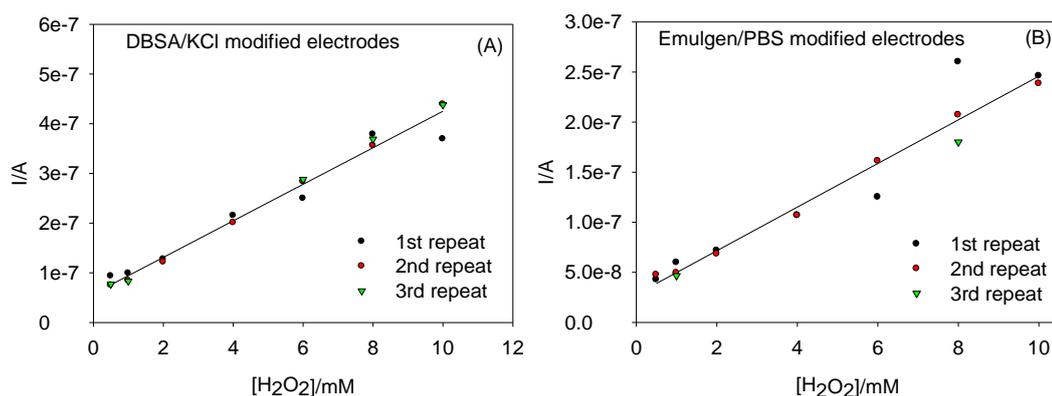
**Fig. 5.21.** Amperometric measurement of H<sub>2</sub>O<sub>2</sub> at 420 s in the presence of assay reagents using A) DBSA/KCl modified electrodes and B) Emulgen B-66/PBS modified electrodes (240 s incubation time).
