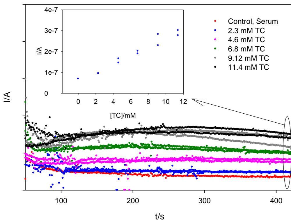
**Fig. 5.28. Amperometric measurement of 0 to 11 mM TC in the presence of 156 U/mL ChEs and 60 U/mL ChOx and after 180 s incubation time. Inset: Biosensor response to 0 to 11 mM TC concentration at 420 s.**
