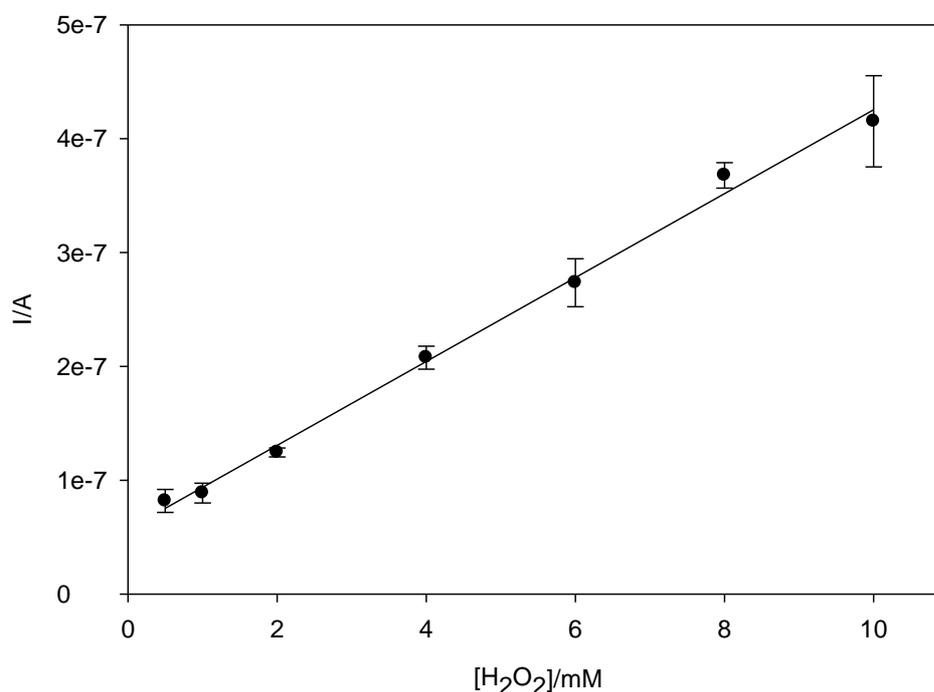
**Fig. 4.10. Chronoamperometric response of modified electrodes to 8 μL of H<sub>2</sub>O<sub>2</sub> (-0.1 V vs Ag/AgCl at 420 s) in the presence of the final assay reagent formulation and delipidated serum at 420 s, (slope=3.7×10<sup>-8</sup> A/mM, r<sup>2</sup>=0.99, RSD=7.2%).**
