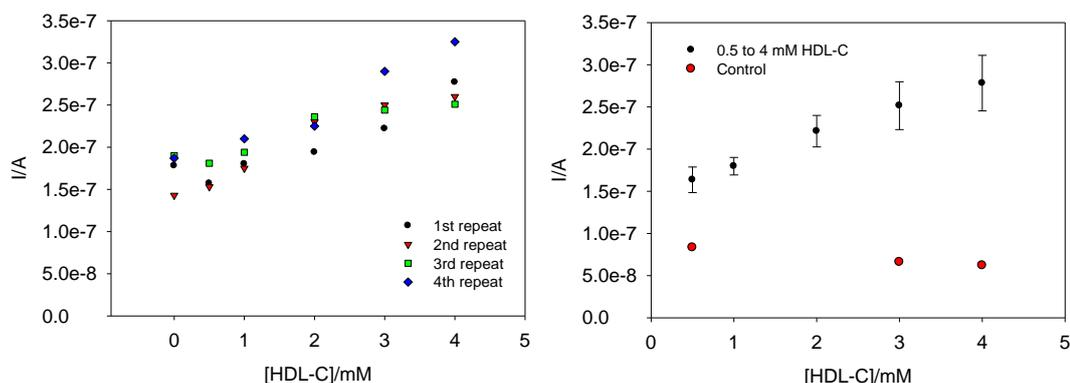
**Fig. 6.19. Amperometric measurement of HDL-C (0.5-4 mM) at -0.1 V vs Ag/AgCl using integrated biosensors with four printed reagent layers containing ChOx (218 U/mL) and ChEs (633 U/mL) in 6% (w/v) Emulgen B-66/PBS and 0.2% (w/v) PVP and PDA (slop= $3.33 \times 10^{-8}$ ,  $r^2=0.993$  and RSD=10.3%;  $n=4$ ), Enzymes-less assay reagent inkjet-print deposited on modified electrode surface was used for control measurement.**
