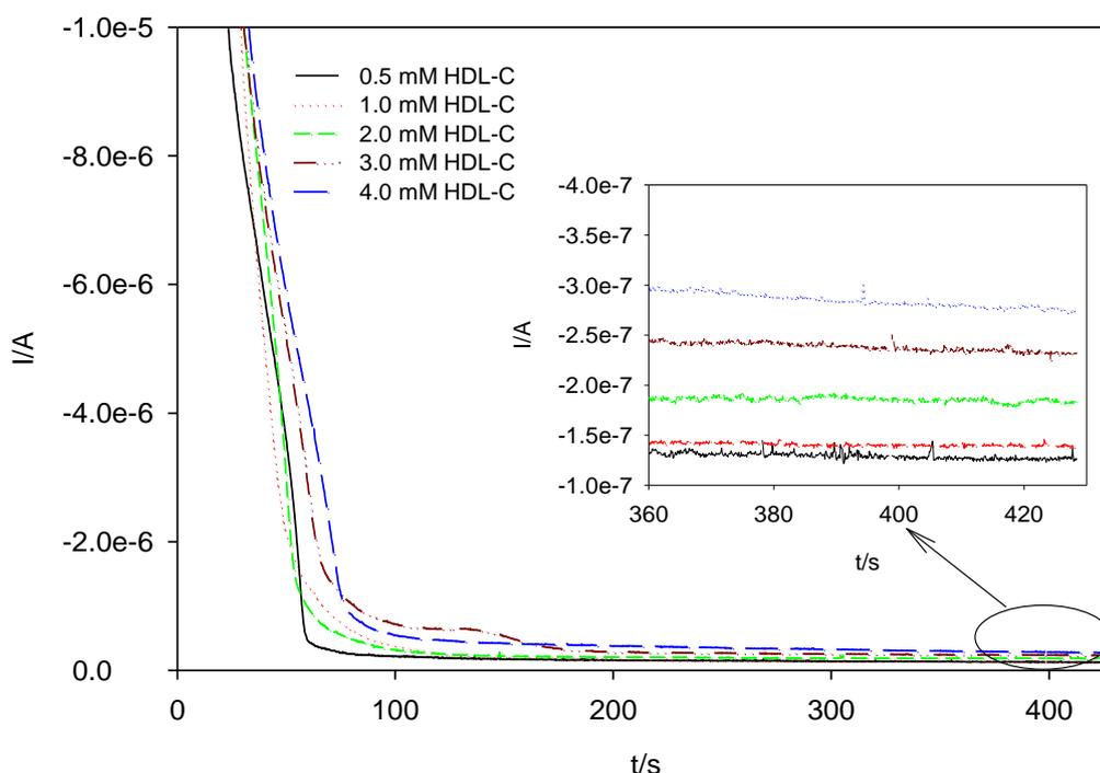
**Fig. 5.8. Chronoamperometric response of encapsulated biosensors to 0 to 4 mM HDL-C in delipidated serum at -0.1V (vs Ag/AgCl). Inset: Detail of biosensors response between 360 and 420 s.**
