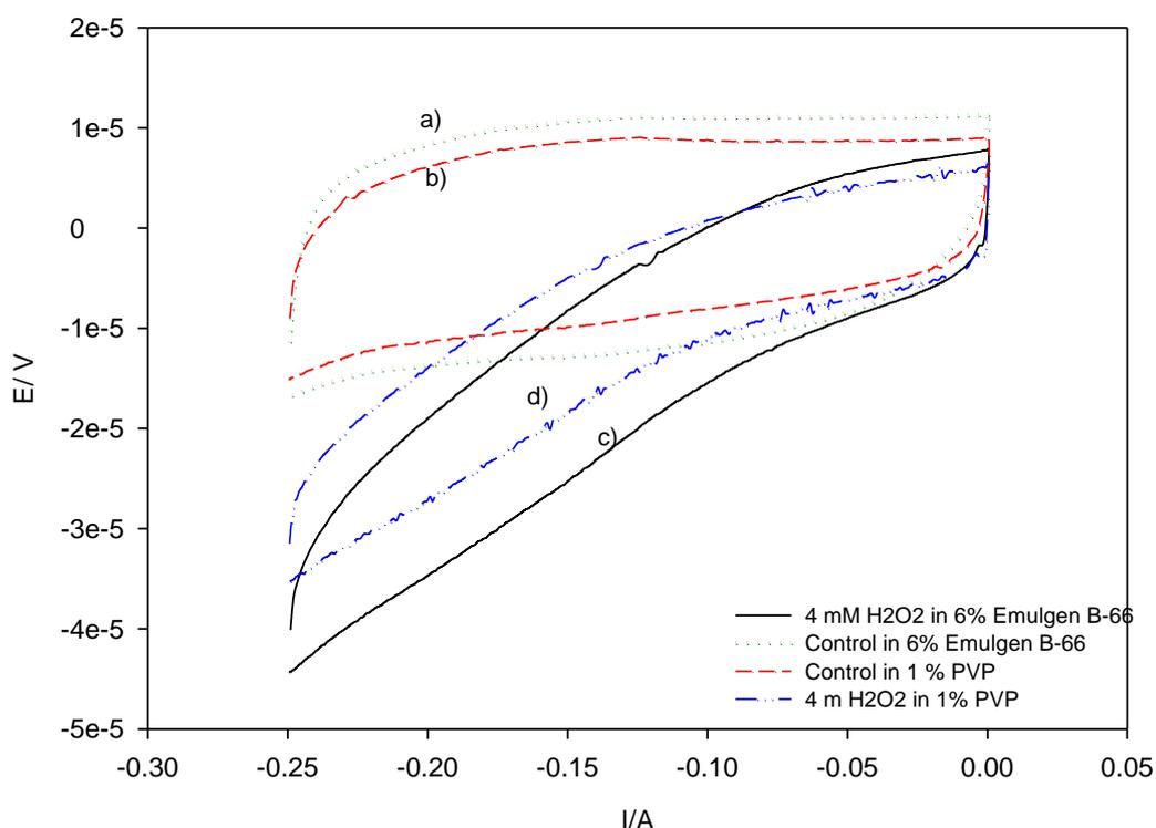
**Fig. 6.12. Cyclic voltammogram of modified electrodes in a) 6% (w/v) Emulgen B-66, b) 0.1% (w/v) PVP, c) 4 mM H<sub>2</sub>O<sub>2</sub> in 6% (w/v) Emulgen B-66 and d) 4 mM H<sub>2</sub>O<sub>2</sub> in 0.1% (w/v) PVP, Delipidated serum was used for control experiments.**
