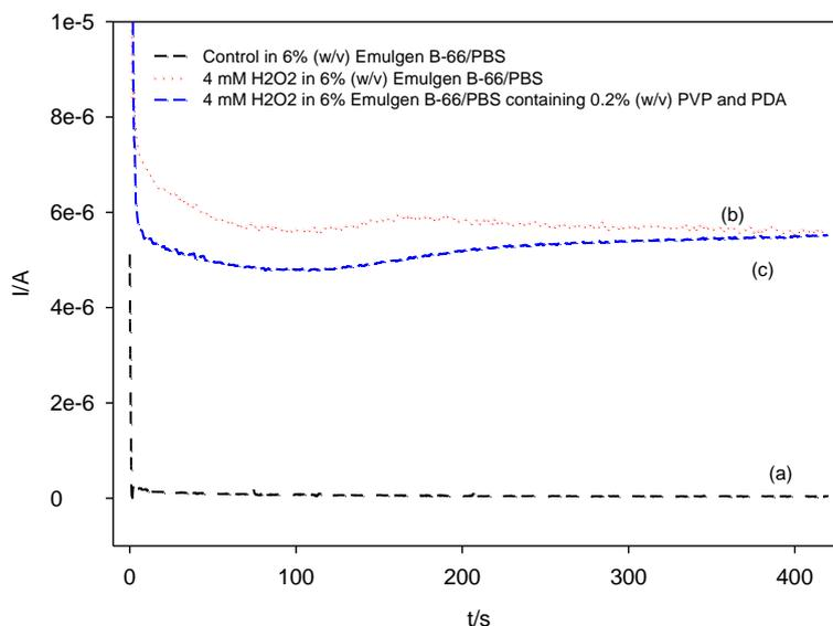
**Fig. 6.14. Amperometric measurement of H<sub>2</sub>O<sub>2</sub> (4 mM) in the absence (b) and the presence (c) of combined 0.2% (w/v) PVP and PDA in 6% (w/v) Emulgen B-66/PBS; Delipidated serum used for control measurement (a) in the absence of combined 0.2% (w/v) PVP and PDA.**
