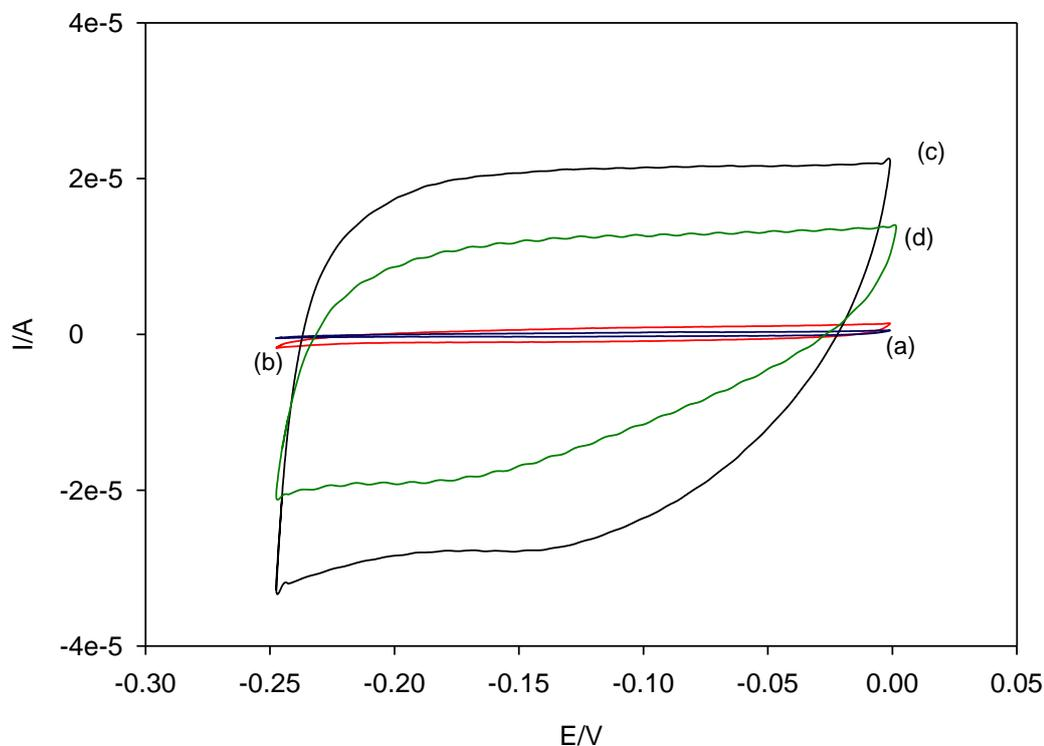
**Fig. 5.15. Cyclic voltammograms of unmodified silver electrode measured in 6% (w/v) Emulgen B-66 using: a) un-modified electrode in PBS, b) electrodes dipped in 6% (w/v) Emulgen B-66/PBS for 180 min, c) drop coated electrode using 3  $\mu\text{L}$  of 6% (w/v) Emulgen B-66/PBS, d) inkjet-printed electrode using 5 layers 6% Emulgen B-66 (1.2  $\mu\text{L}$ )**
