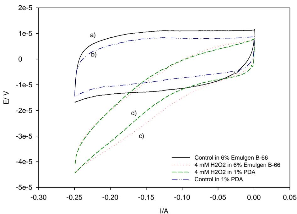
**Fig. 6.10.** Cyclic voltammogram of modified electrodes in a) 6% (w/v) Emulgen B-66, b) 1% (w/v) PDA, c) 4 mM  $H_2O_2$  in 6% (w/v) Emulgen B-66 and d) 4 mM  $H_2O_2$  in 1% (w/v) PDA, delipidated serum was used for control experiments.
