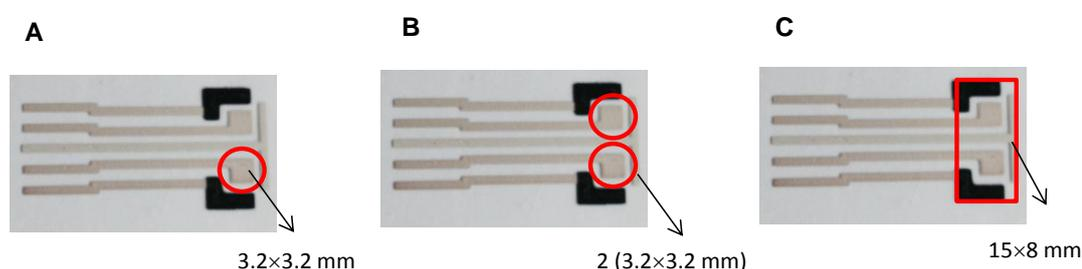
**Fig. 2.6. Schematic showing patterns of printing used for the deposition of assay reagent formulation. A: 3.2  $\times$  3.2 mm single silver working electrode, B: 3.2  $\times$  3.2 mm on two working electrodes and C: 15  $\times$  8 mm across dual three-electrode cells.**
