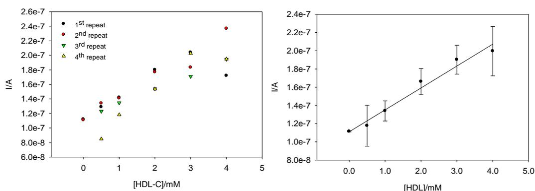
**Fig. 6.6. Chronoamperometric measurement (-0.1 V vs Ag/AgCl) of HDL-C using encapsulated HDL-C biosensors using 2 layers of assay reagent inkjet-printed on 15 × 8 mm of Emulgen/PBS modified electrode, after 240 s incubation at room temperature, (slope= $2.06 \times 10^{-8} \text{ A/mM}$ ,  $r^2=0.952$ ,  $n=4$ ).**
