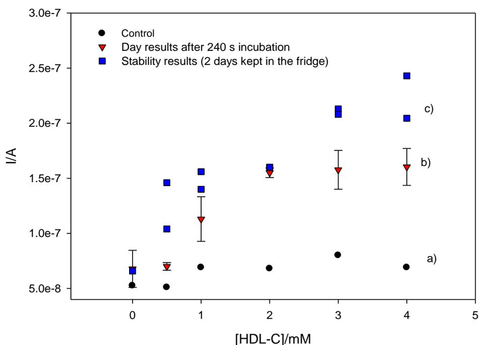
**Fig. 6.16. Amperometric measurement (-0.1 V vs Ag/agCl) of HDL-C at 420 s using the integrated biosensor after 240 s incubation: a) control experiment in the absence of the enzymes, b) response from biosensors tested on the same day as fabrication (slope=  $2.57 \times 10^{-8}$ ,  $r^2 = 0.825$ , (n=3)) and c) after two days storage at 2-8 °C (slope=  $3.32 \times 10^{-8}$ ,  $r^2 = 0.849$ , (n=2))**
