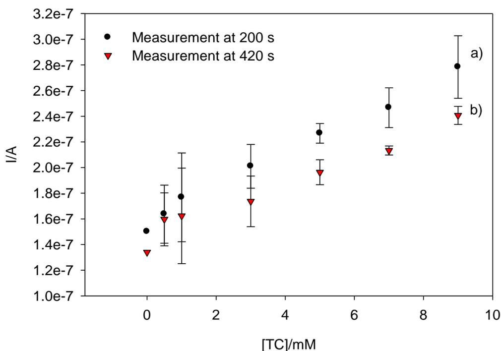
**Fig. 6.26. Amperometric measurement of TC using integrated biosensors with unmodified silver paste electrodes (-0.1 V vs Ag/AgCl) at a) 200 s (slope= $1.34 \times 10^{-8}$ ,  $r^2=0.99$  and RSD=10% (n=3)) and b) 420 s (slope= $9.38 \times 10^{-9}$  A/mM and  $r^2$  of 0.982, RSD=9.5%; n=3).**
