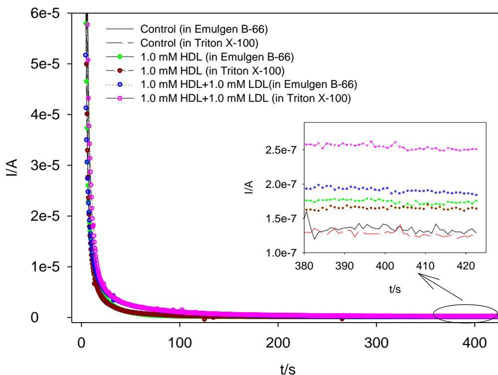
**Fig. 5.4. Chronoamperometric measurement of 1 mM HDL-C in the presence and absence of 1 mM LDL-C at -0.1 V (vs Ag/AgCl), Emulgen B-66 and Triton X-100 were used for HDL-C and TC measurements, respectively. Inset: Detail of biosensor responses between 380 and 420 s.**
