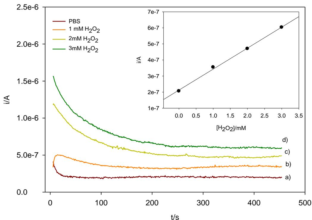
**Fig. 4.3. Chronoamperometric responses of encapsulated modified Ag SPEs measured at -0.1V (vs Ag/AgCl) in a) 0.1 M PBS pH 6.8, b) 1 mM  $\text{H}_2\text{O}_2$ , c) 2 mM  $\text{H}_2\text{O}_2$  and d) 3 mM  $\text{H}_2\text{O}_2$ ; Inset: Plot of the current vs  $\text{H}_2\text{O}_2$  concentration at  $t=300$  s.**
