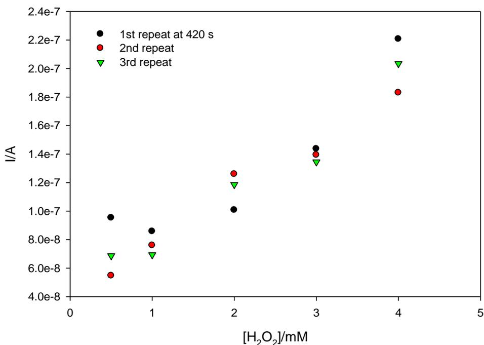
**Fig. 6.5. Chronoamperometric measurement (-0.1 V vs Ag/AgCl) of H<sub>2</sub>O<sub>2</sub> using encapsulated HDL-C biosensors using 10 layers of inkjet-printed assay reagent deposited on both silver electrode, after 240 s incubation at room temperature, (slope= $3.62 \times 10^{-8}$  A/mM,  $r^2=0.956$ ).**
