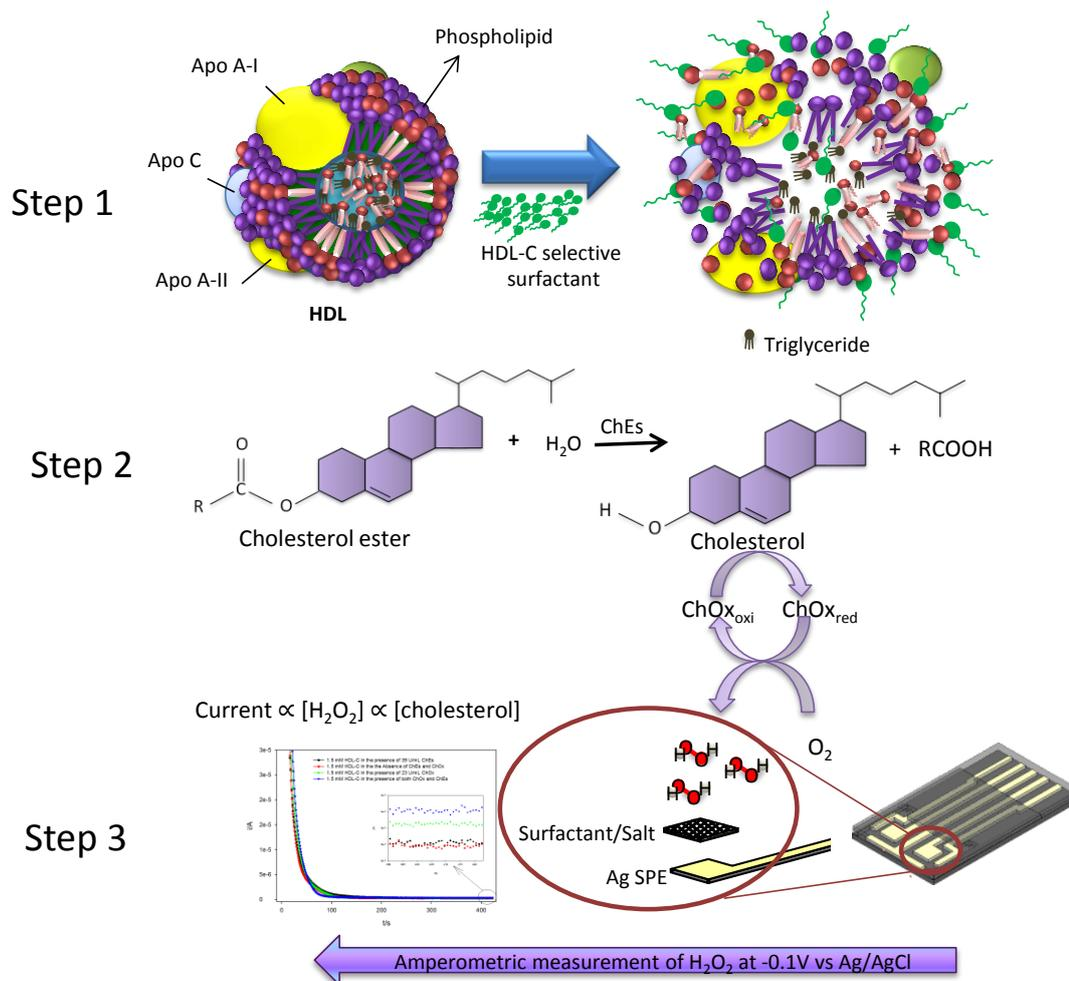
**Fig. 2.4. General approach to the amperometric measurement of HDL-C using externally added reagents. Step 1 and 2: externally addition of assay reagent containing HDL-C selective surfactant solubilises the HDL which allows access to cholesterol esterase (ChEs) and cholesterol oxidase (ChOx) presents in the reagent at room temperature. Step 3: The generated H<sub>2</sub>O<sub>2</sub> can then be measured using modified electrodes at -0.1 V vs. Ag/AgCl which is measured at 420 s.**
