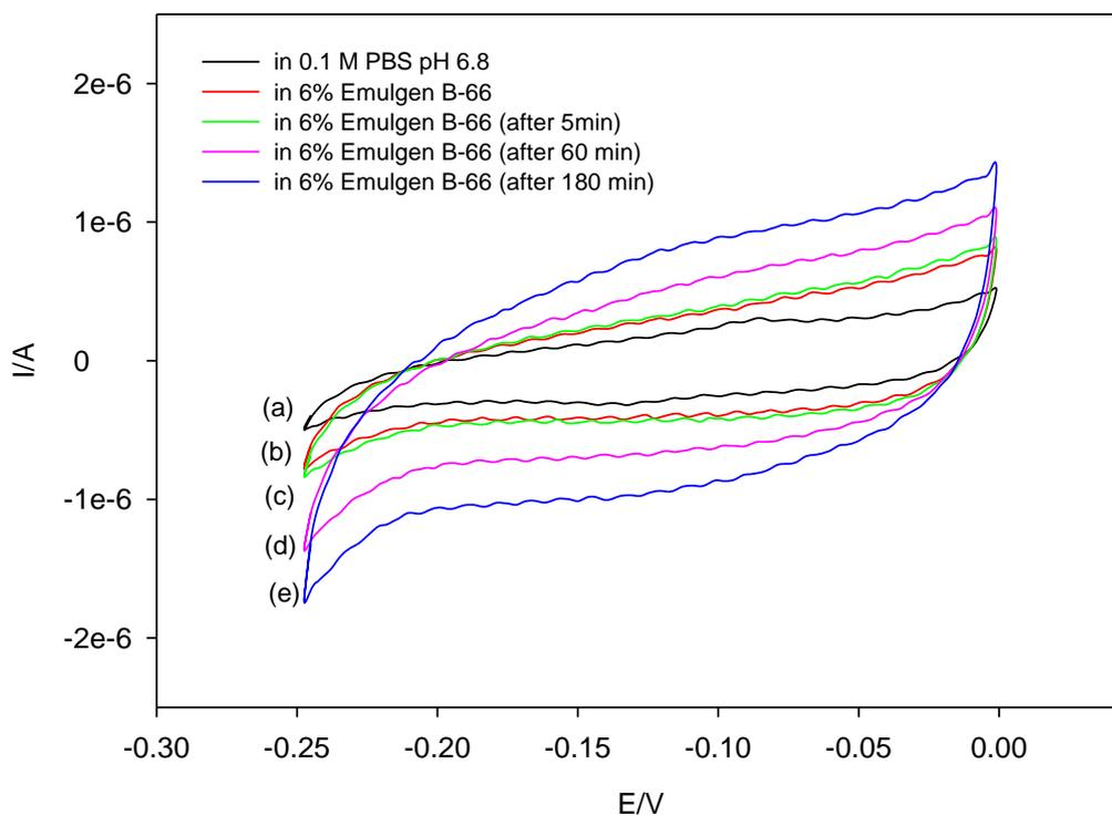
**Fig. 5.14. Cyclic voltammograms of a) unmodified silver electrodes measured in PBS following exposure to 6% (w/v) Emulgen B-66/PBS for b) 0 min, c) 5 min, d) 60 and e) 180 min.**
