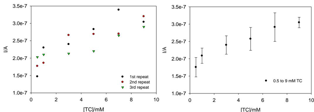
**Fig. 6.24. Amperometric measurement of TC (-0.1 V vs Ag/AgCl) using the integrated biosensor containing ChEs (1566 U) and ChOx (582 U) in 1.5 mL of 0.25% (v/v) Triton X-100 containing 0.2% (w/v) PVP and PDA after 240 s incubation at 420 s (slope= $1.415 \times 10^{-8}$  A/mM and  $r^2=0.949$ , RSD=11.6% n=3).**
