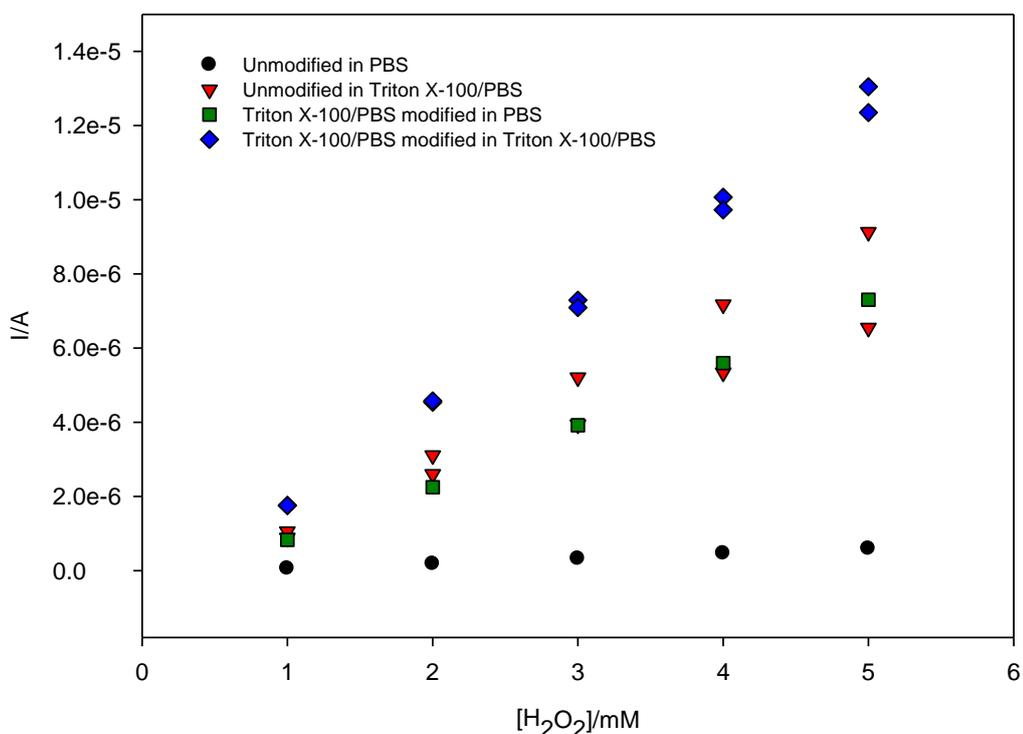
**Fig. 5.30. Amperometric measurement  $\text{H}_2\text{O}_2$  in stirred solution at 420 s using unmodified and Triton X-100/PBS modified electrodes in both PBS and 0.5% (v/v) Triton X-100/PBS solution.**
