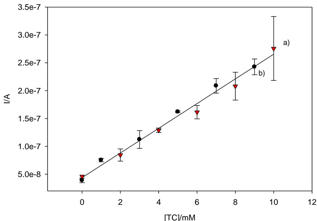
**Fig. 6.22.** Biosensor response to TC in delipidated serum at -0.1 V (vs Ag/AgCl) after 420 s using externally addition of assay reagent a) (triangles) in the absence of PVP and PDA (slope= $2.24 \times 10^{-8}$  A/mM,  $r^2 = 0.984$  and RSD=10.8%; n=3) b) (circles) in the presence of stabilizers (slope= $2.25 \times 10^{-8}$  A/mM,  $r^2 = 0.994$  and RSD=7.0%; n=3).
