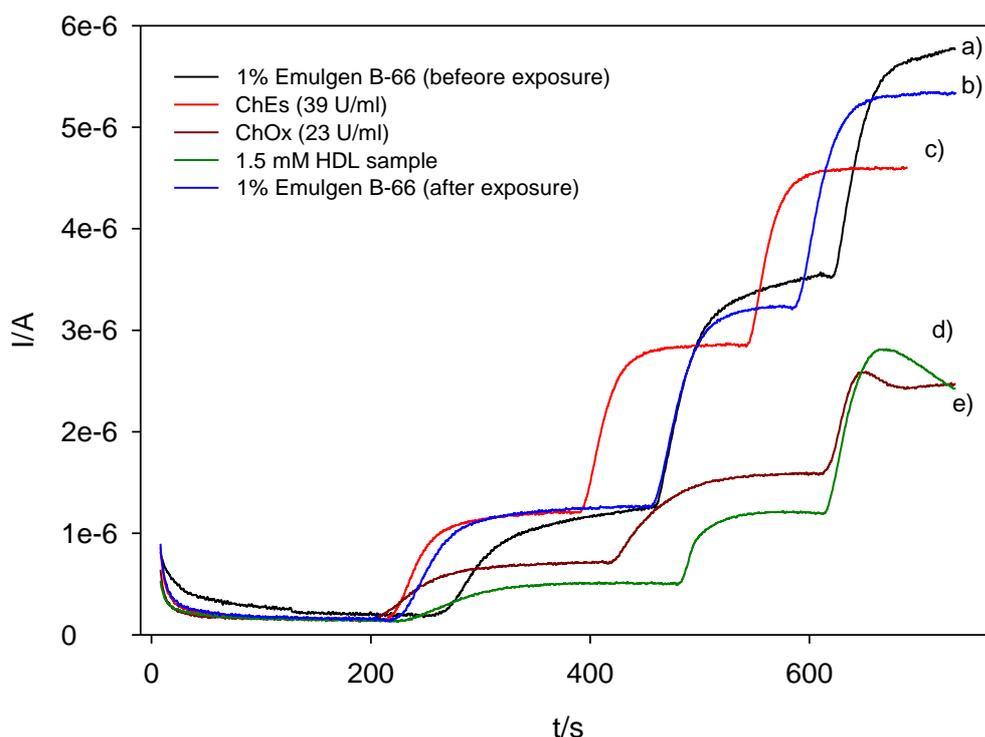
**Fig. 4.7.** Amperometric response of sensors to H<sub>2</sub>O<sub>2</sub> (0.5 to 1.5 mM) in stirred solution containing 1% (w/v) Emulgen B-66: a) before exposure and; b) after exposure to a solution of ChEs (39 U/mL), ChOx (23 U/mL) and serum containing 1.5 mM HDL-C; c) in the presence of ChEs (39 U/mL); d) in the presence of serum containing 1.5 mM HDL-C; e) in the presence of ChOx (23 U/mL).
