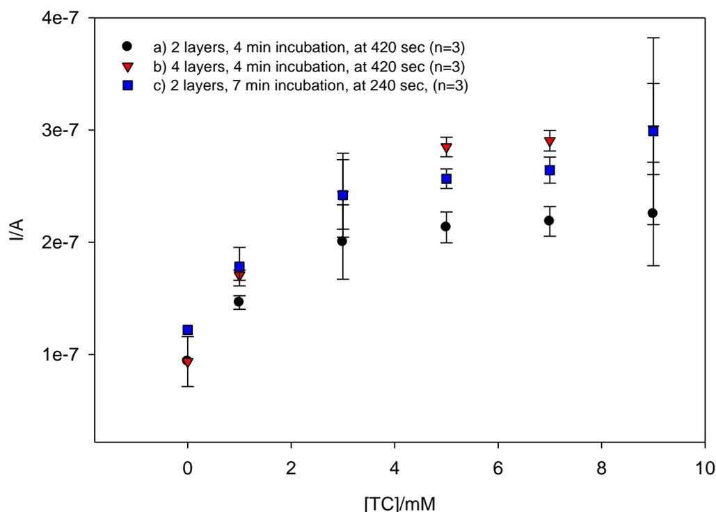
**Fig. 6.23. Amperometric measurement of TC using the integrated biosensor (-0.1V vs Ag/AgCl) at 420 s using: two printed reagent layers a) after 240 s incubation (slope= $1.31 \times 10^{-8}$  A/mM and  $r^2=0.772$ ) and c) after 420 s incubation (slope= $1.73 \times 10^{-8}$  A/mM and  $r^2=0.864$ ) and also b) using four reagent layers after 240 s incubation (slope= $2.139 \times 10^{-8}$  A/mM and  $r^2=0.864$ ).**
