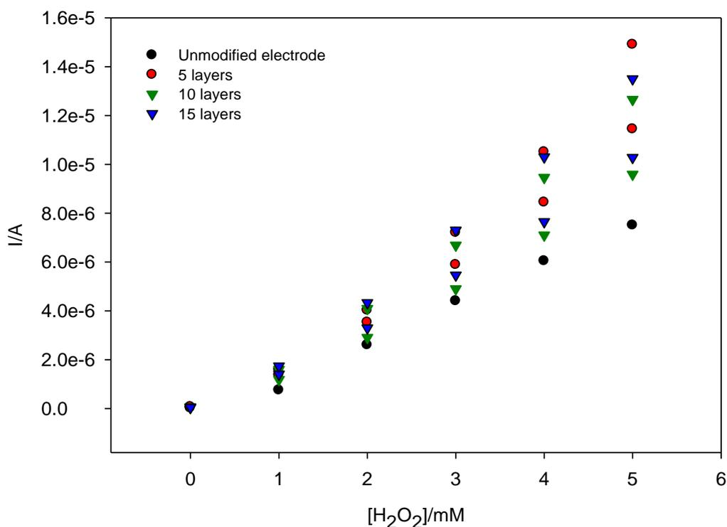
**Fig. 5.33. Amperometric measurement of H<sub>2</sub>O<sub>2</sub> in 0.5% (v/v) Triton X-100/PBS in stirred batch cell at -0.1 V vs. Ag/AgCl using unmodified electrodes, and electrodes modified with 5, 10 and 15 inkjet-printed layers of Triton/PBS.**
