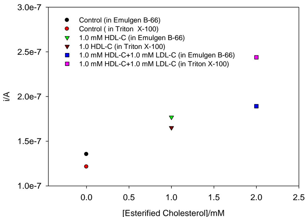
**Fig. 5.5. Chronoamperometric response at 420 s (-0.1 V (vs Ag/AgCl)) to 1 mM HDL-C in the presence and the absence of 1 mM LDL-C using selective and non-selective surfactants.**
