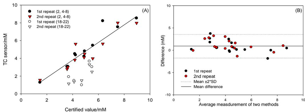
**Fig. 5.36. Correlation of total cholesterol in serum measured by the biosensor and certified value (slope= 1.07,  $r=0.87$ ). Inset: plot of differences versus average with 95% limits of agreement**
