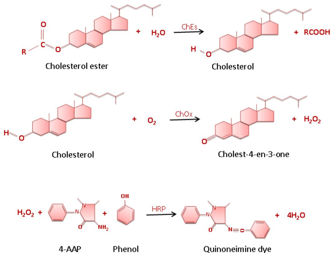
**Fig. 1.4. Spectrophotometric measurement of cholesteryl ester and cholesterol using cholesterol esterase (ChEs) and cholesterol oxidase (ChOx). The generation of  $H_2O_2$  is detected using horseradish peroxidase (HRP) in the presence of 4-aminoantipyrine (4-APP) and Trinder's dye (phenol), generating a quinoneimine dye, the optical density of which is measured at 500 nm (Allain *et al.*, 1974).**
