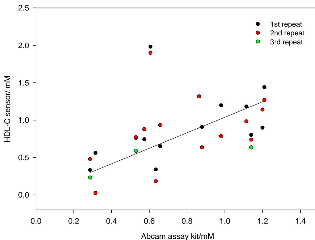
**Fig. 5.24. Correlation of HDL-C in serum measured by the biosensor and the Abcam assay kit (n=13) (slope= 0.87, r=0.76).**
