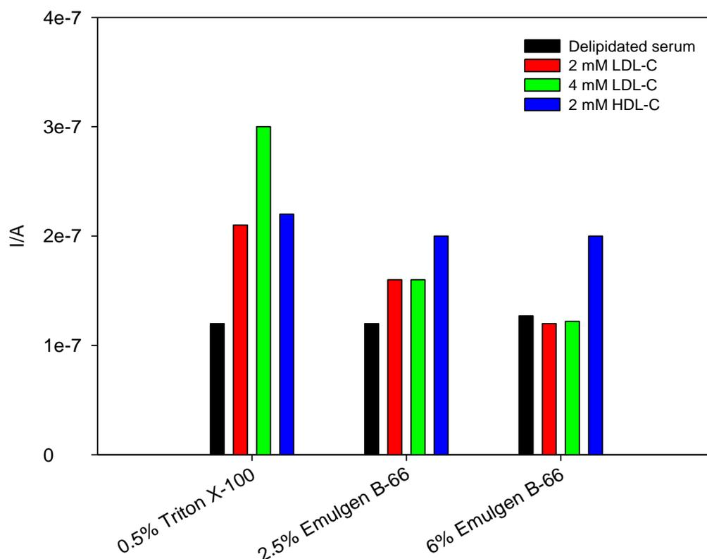
**Fig. 5.7. Biosensor responses of 2 mM HDL-C, 2 and 4 mM LDL-C in the presence of HDL-C selective and non-selective surfactants at 420 s and after 180 s incubation time.**
