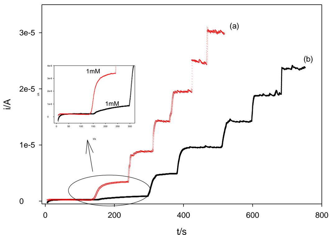
**Fig. 4.4.** Effect of Emulgen B-66 on the response of the modified electrode to the reduction of  $\text{H}_2\text{O}_2$  ( $-0.1$  V vs. Ag/AgCl). a) 1% (w/v) Emulgen B-66 in 0.1 M PBS pH 6.8; b) 0.1 M PBS pH 6.8. Inset: Detail of biosensor responses between 0 and 300 s.
