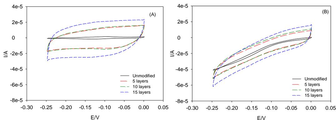
**Fig. 5.32. Cyclic voltammograms of unmodified electrodes and those modified with 5, 10 and 15 inkjet-printed layers in: A) 0.5% (v/v) Triton X-100/PBS solution and B) 5 mM H<sub>2</sub>O<sub>2</sub>.**
