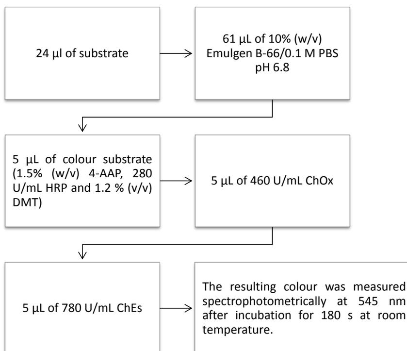
**Fig. 2.3. Flow diagram for spectrophotometric assay methodology developed at room temperature for this work using 96 well microtitre plates**
