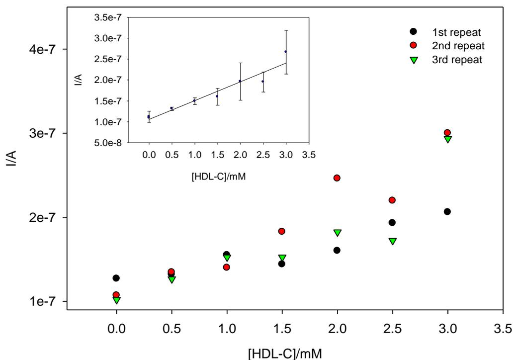
**Fig. 5.12.** HDL-C biosensor response to delipidated serum containing 0 to 3 mM HDL-C and 4 mM LDL-C. Inset: calibration curve (slope:  $4 \times 10^{-8}$  A/mM,  $r^2=0.93$ ,  $n=3$ ).
