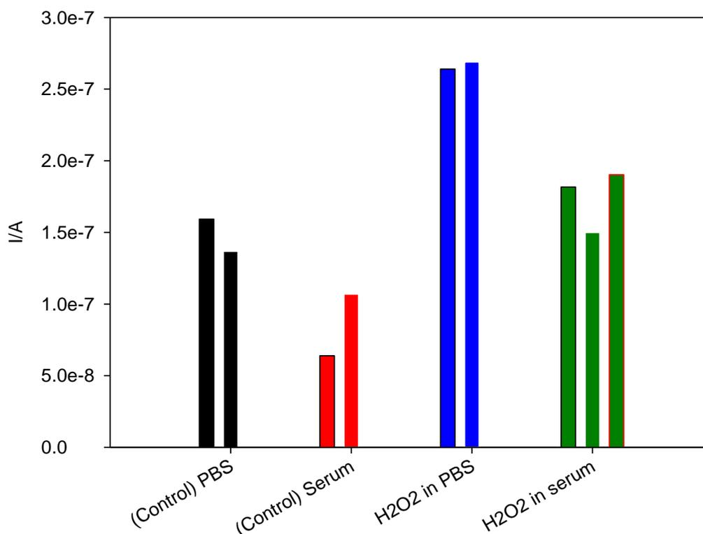
**Fig. 4.9. Amperometric measurement of 3 mM H<sub>2</sub>O<sub>2</sub> prepared in PBS compared to the one prepared in delipidated serum at 420 s.**
