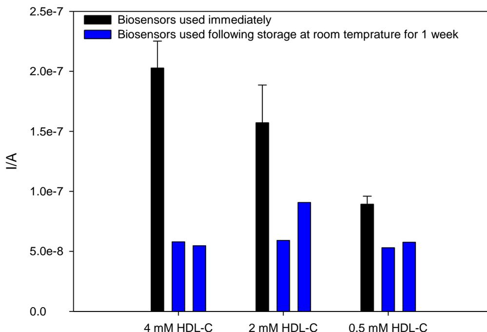
**Fig. 6.9. Amperometric measurement of HDL-C (-0.1 V vs Ag/AgCl) using the developed biosensor used on the day of fabrication (black) and after one week in a desiccator at room temperature.**
