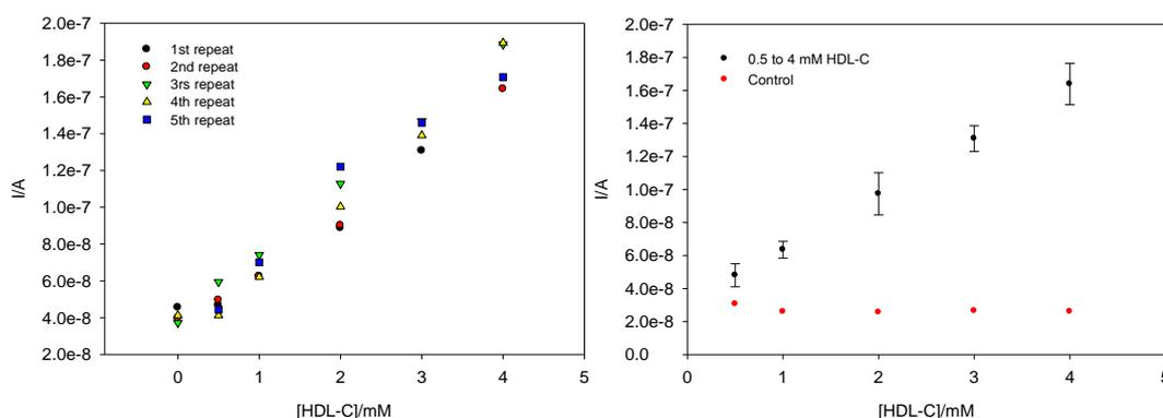
**Fig. 5.22. Biosensor response to HDL-C in delipidated serum at -0.1 V (vs Ag/AgCl). a) Biosensor controls in the absence of ChEs and ChOx; b) Biosensor containing 6% (w/v) Emulgen B-66, 39 U/mL ChEs and 23 U/mL ChOx; (slope= $3.32 \times 10^{-8}$ ,  $r^2=0.999$ ,  $n=5$ ).**
