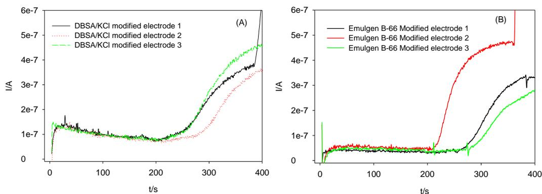
**Fig. 5.20. Background current and the current observed for 0.5 mM  $\text{H}_2\text{O}_2$  in 6% (w/v) Emulgen B-66/PBS solution using: A) DBSA/KCl modified electrodes and B) Emulgen B-66/PBS modified electrodes (Stirred batch experiment).**
