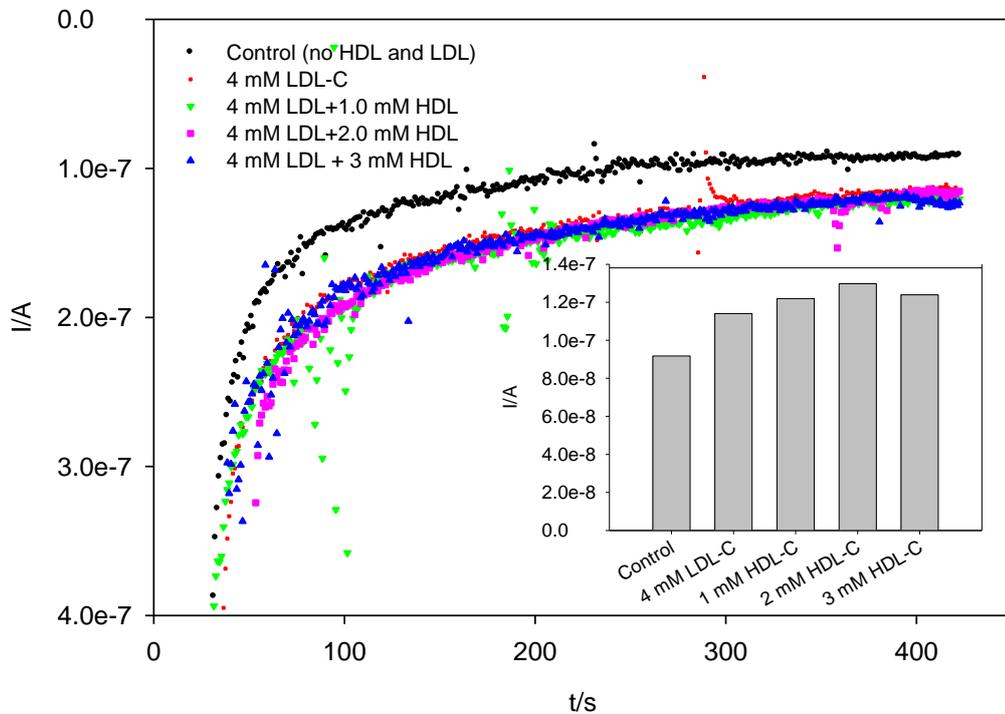
**Fig. 5.11. Chronoamperometric measurement of FC present in delipidated serum containing 0 to 3 mM HDL-C and 4 mM LDL-C. Inset: Biosensor response at 420 s in delipidated serum was used as control.**
