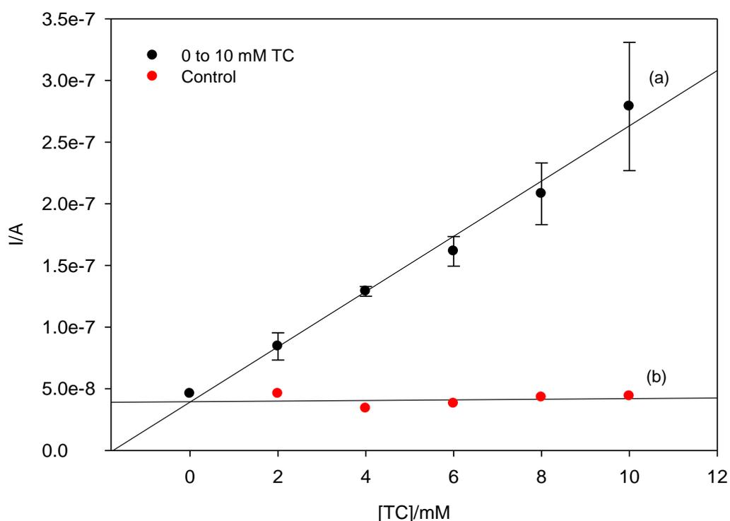
**Fig. 5.34. Biosensor response to total cholesterol in delipidated serum at -0.1 V (vs Ag/AgCl) after 420 s. a) modified electrode using externally mixed reagents containing 0.5% (v/v) Triton X-100, 156 U/mL ChEs and 60 U/mL ChOx; (slope= $2.24 \times 10^{-8}$  A/mM,  $r^2=0.984$  and RSD=10.8%; n=3); b) controls in the absence of ChEs and ChOx.**
