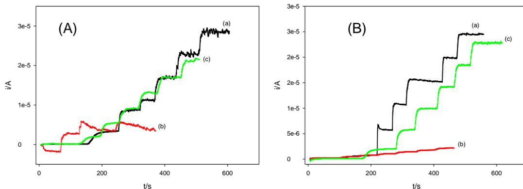
**Fig. 4.5. Amperometric response of the modified electrodes to  $\text{H}_2\text{O}_2$  (0-6 mM) in 1% (w/v) Emulgen B-66 prepared in (A) 50 mM MOPS pH 7.3 and (B) 0.1 M Tris-HCl pH 7.0. (a) Response in 0.1 M PBS pH 6.8 before testing in MOPS/Tris; (b) responses in MOPS/Tris; (c) Response in 0.1 M PBS after testing in MOPS/Tris.**
