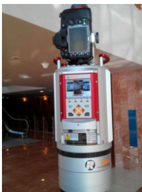
Figure 3: 3D scanning/photogrammetry devices used in our study: the RIEGL VZ-400 TLS equipped with the Nikon D600 digital camera.
