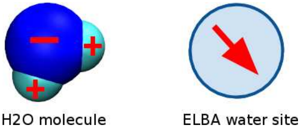
Figure 1: Water coarse-graining. The left image depicts a single water molecule; the oxygen atom (blue) bears a negative charge (red “-” sign), while the two hydrogen atoms (cyan) bear positive charges (red “+” signs). The right image depicts an ELBA coarse-grained water site; the red arrow represents a permanent electrical point dipole.
