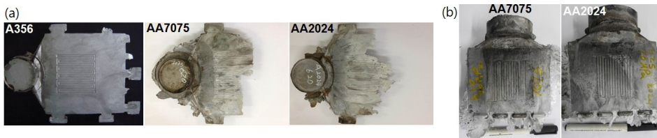
Fig. 14. Thixoforged thin plates (a) horizontal filling die and (b) vertical filling die.
